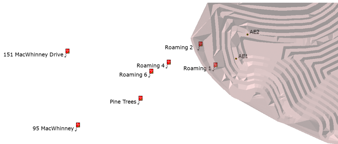
Figure 1 Vibration monitoring locations with seed holes AE1, AE2
