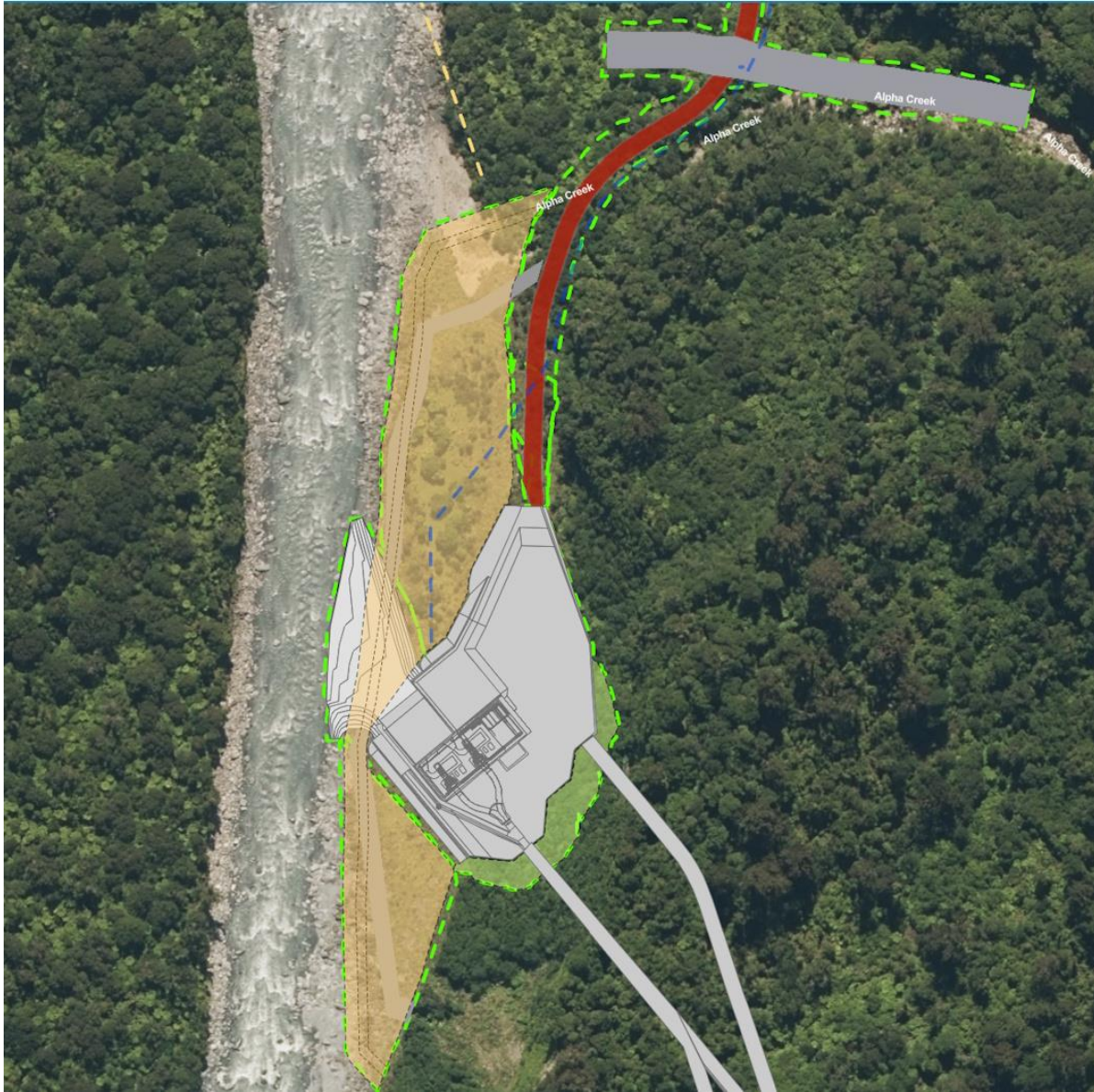
Figure 3. Power Station general layout showing most works located in an open, sparsely wooded alluvial flat. The transmission line and access road corridor (to the top of the figure at Alpha Creek) is within the start of regenerating kamahi forest.
