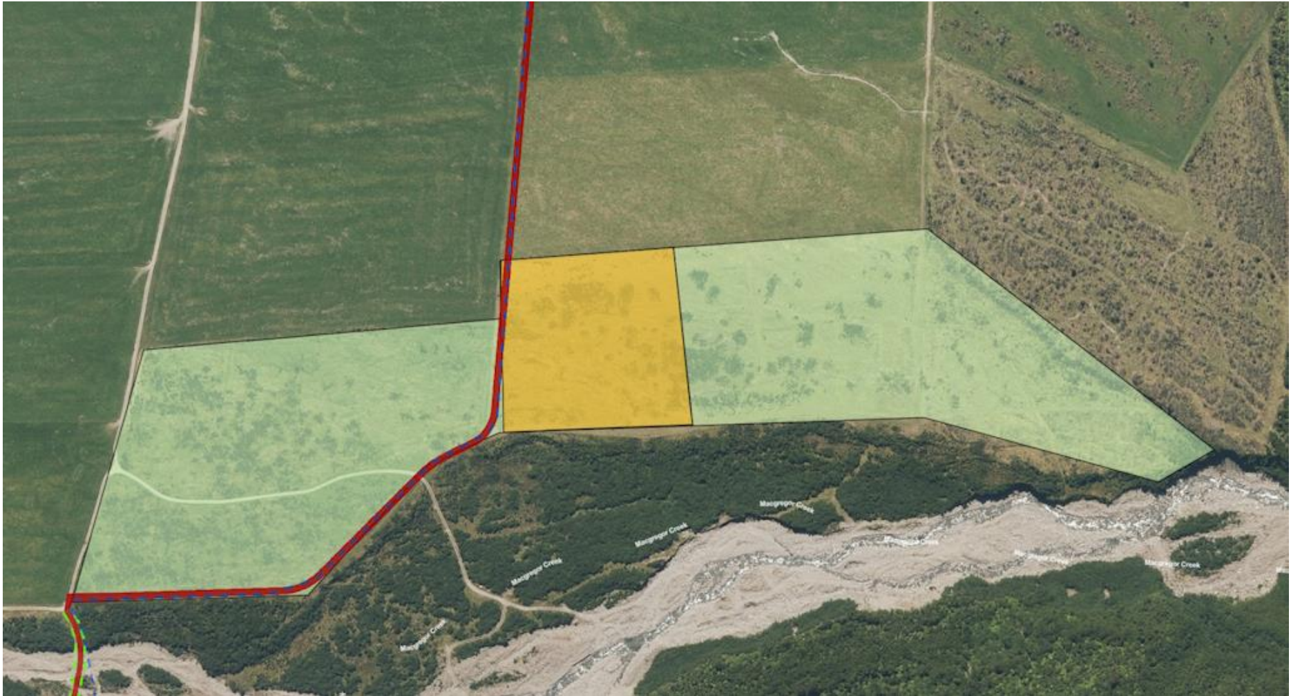
Figure 5. Spoil disposal (shaded green) and construction staging Area 3 (shaded yellow) on the true right bank of Macgregor Creek. The red dotted line is the main access through the farm to the site.
