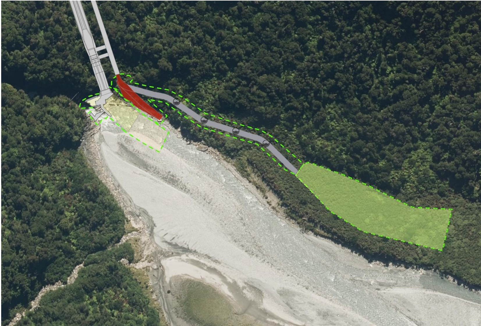
Figure 2. Headworks general layout, with the temporary access road (grey line) and construction laydown area (green shaded polygon) to the east of the portal as the main features that may support native lizards. The extent of proposed construction disturbance/ vegetation clearance is shown as the hashed green line.
