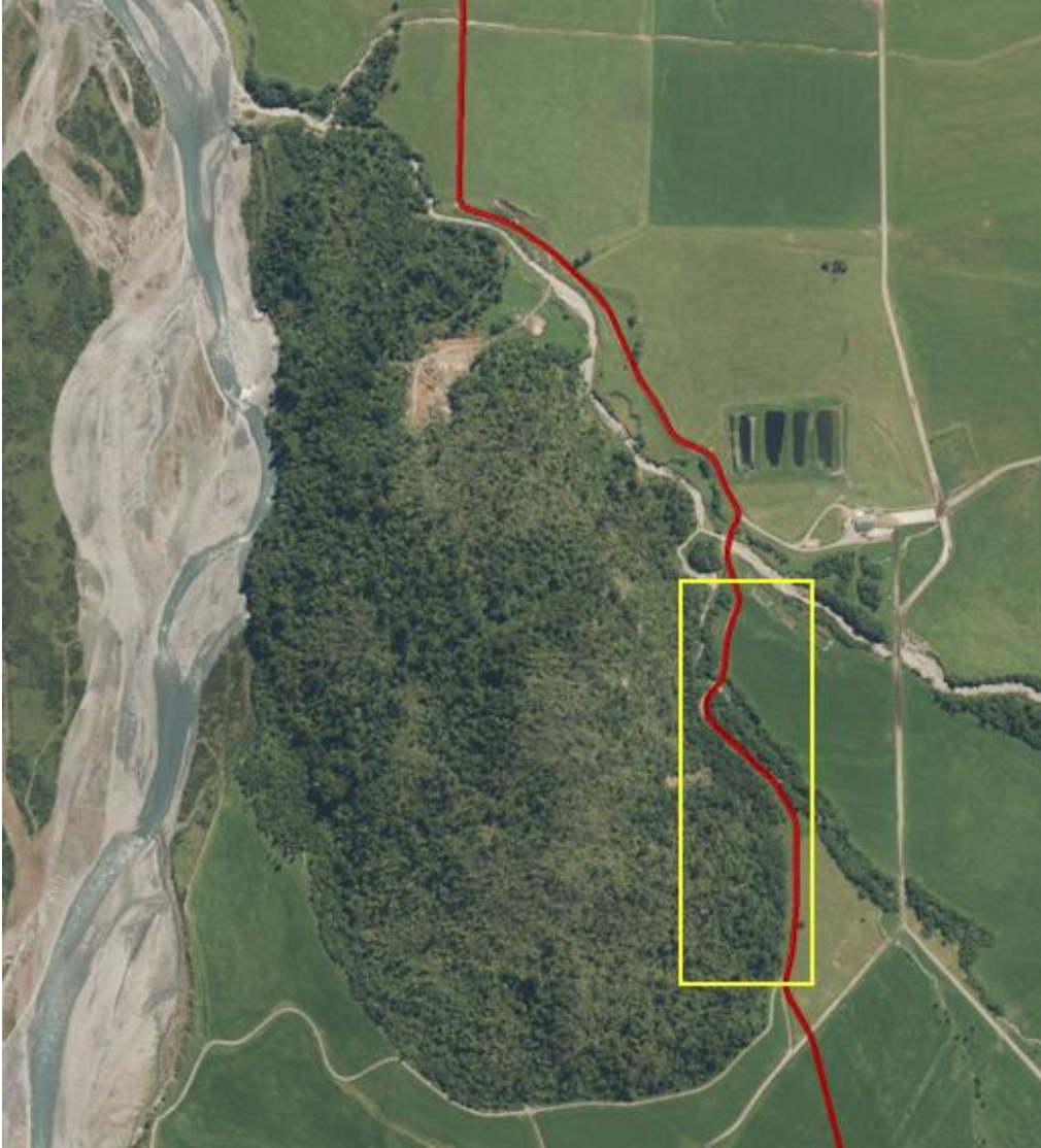
Figure 6. The Doughboy (forested hill) with proposed main access road shown in red, which follows an existing farm road. The upgrade of the road from a 4 m farm track to 10 m wide access track along its current alignment (red line), and the addition of a transmission line (not shown on figure) will involve works within a portion of the eastern side of the Doughboy (generally, the yellow box) and this may require some limited woody vegetation clearance, as well as clearance along the existing rank grass shoulder.
