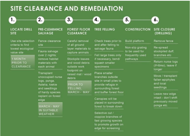
Figure 11-112: General process for vegetation remediation alongside drill site / vent raise site establishment and closure
