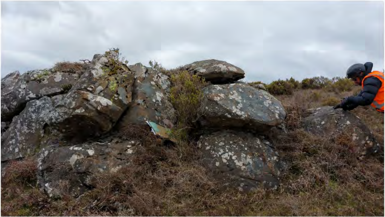
Figure 9: Photo of natural exposure of moderately strong to strong sandstone boulders ('blue-rock') on the strike-ridge at the south end of Jedburgh Station (just north of WTG JED-28) (Oct. 2022).
