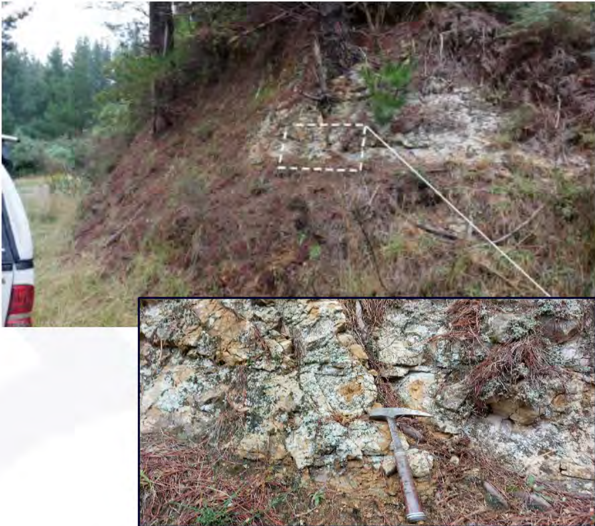
Figure 8: Photo of Venlaw Forest road cut, waypoint 'OC-X2'. Exposure of 'lower-strength' bedrock consisting of very weak to weak sandstone with closely to very closely spaced joint sets – exposed in an over 4m high, moderately inclined cut slope (dashed area showing enlargement photo below).
