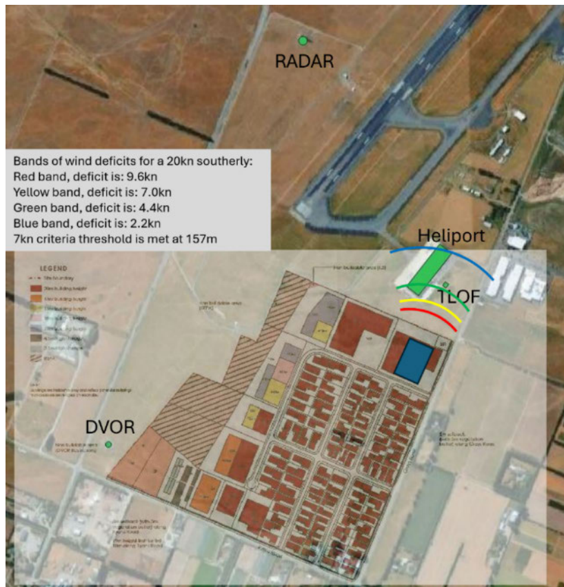
Figure 17 Wind shear from Lot 121 given design of 16m X 80m X 125m (HxWxD)
