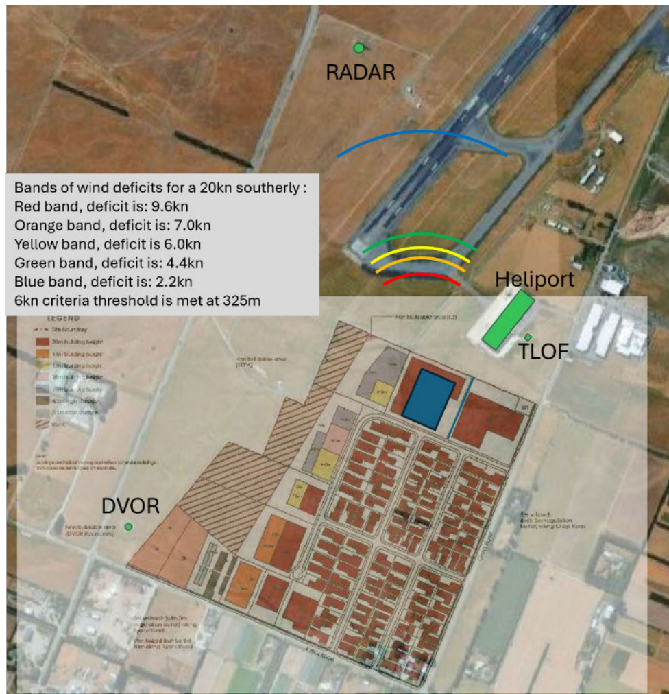
Figure 15: Lot 122 wind shear given a southerly wind and building design of 20m X 100m X 140m (HxWxD)
