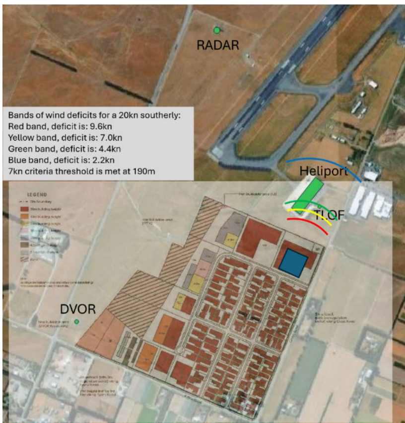
Figure 19 Wind shear from Lot 121 given design of 16m X 100m X 100m (HxWxD)
