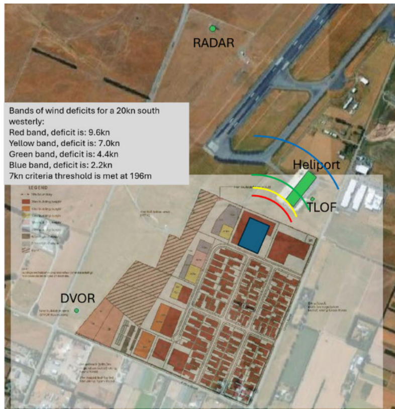
Figure 20 Wind shear from Lot 122 given design of 20m X 100m X 140m (HxWxD)
