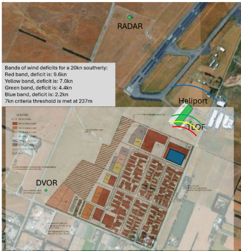
Figure 18 Wind shear from Lot 121 given design of 16m X 125m X 80m (HxWxD)
