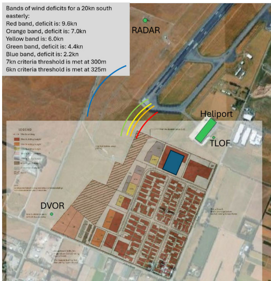
Figure 14 Lot 122 wind shear given an south-easterly wind and building design of 20m X 100m X 140m (HxWxD)
