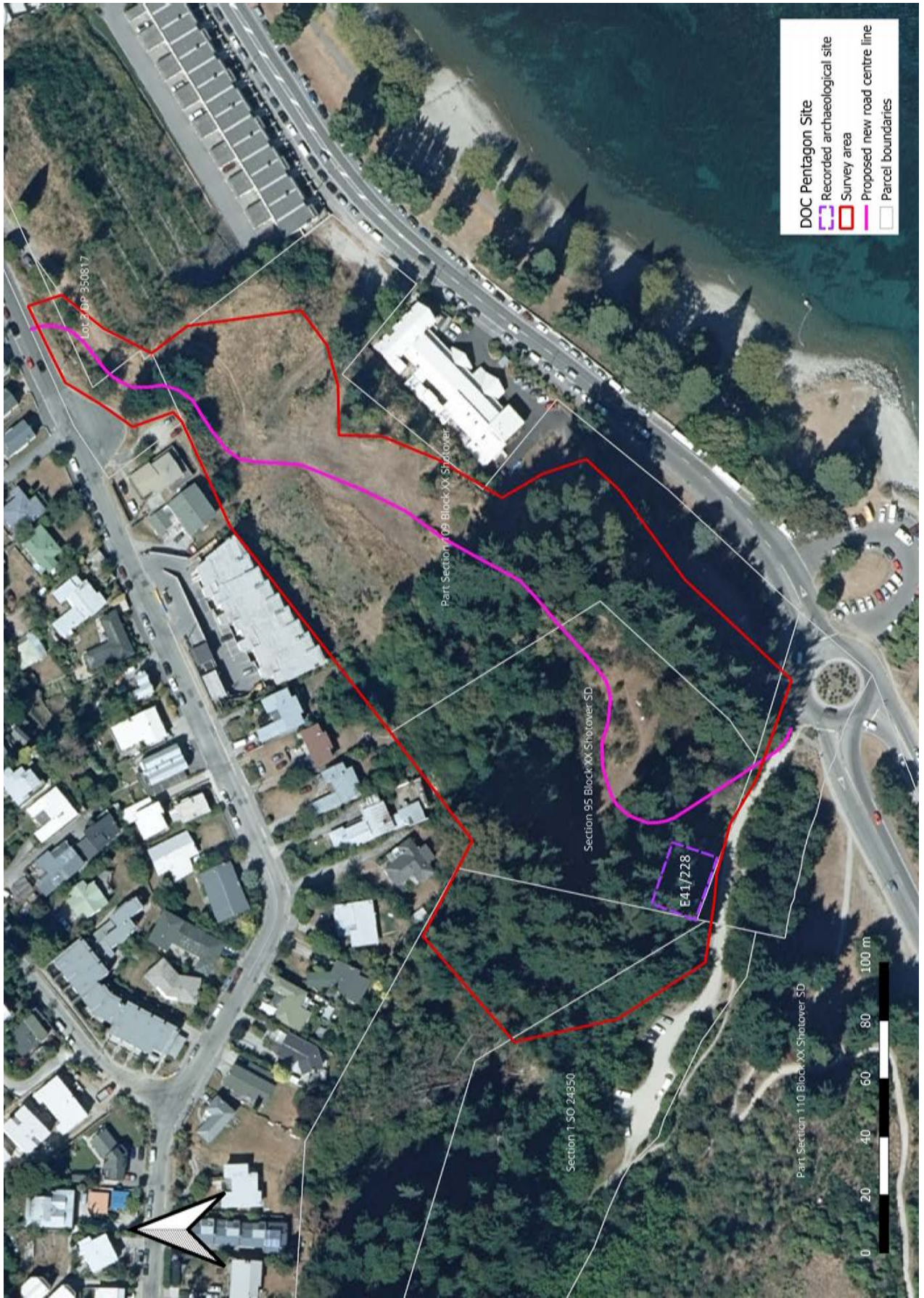
Figure 1A. Full sized map showing tree survey boundaries and location of the centre-line of proposed road.
