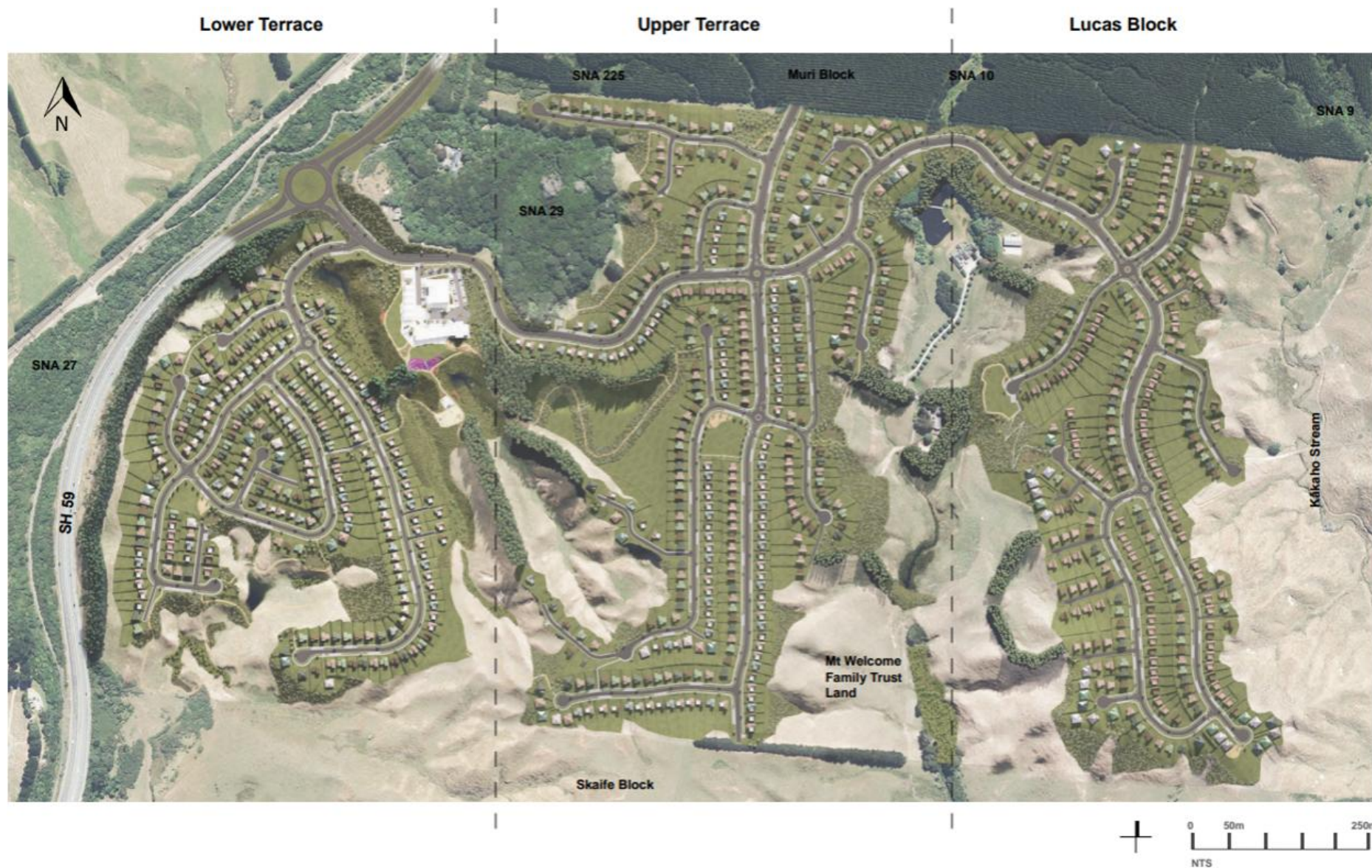
Figure 2. Indicative site plan of the Mt Welcome development project area showing the proposed roads and sections on the Lower Terrace (western extent), Upper Terrace (middle extent), and Lucas Block (eastern extent). Source: Mt Welcome Concept Masterplan 020524 Classic Developments.
