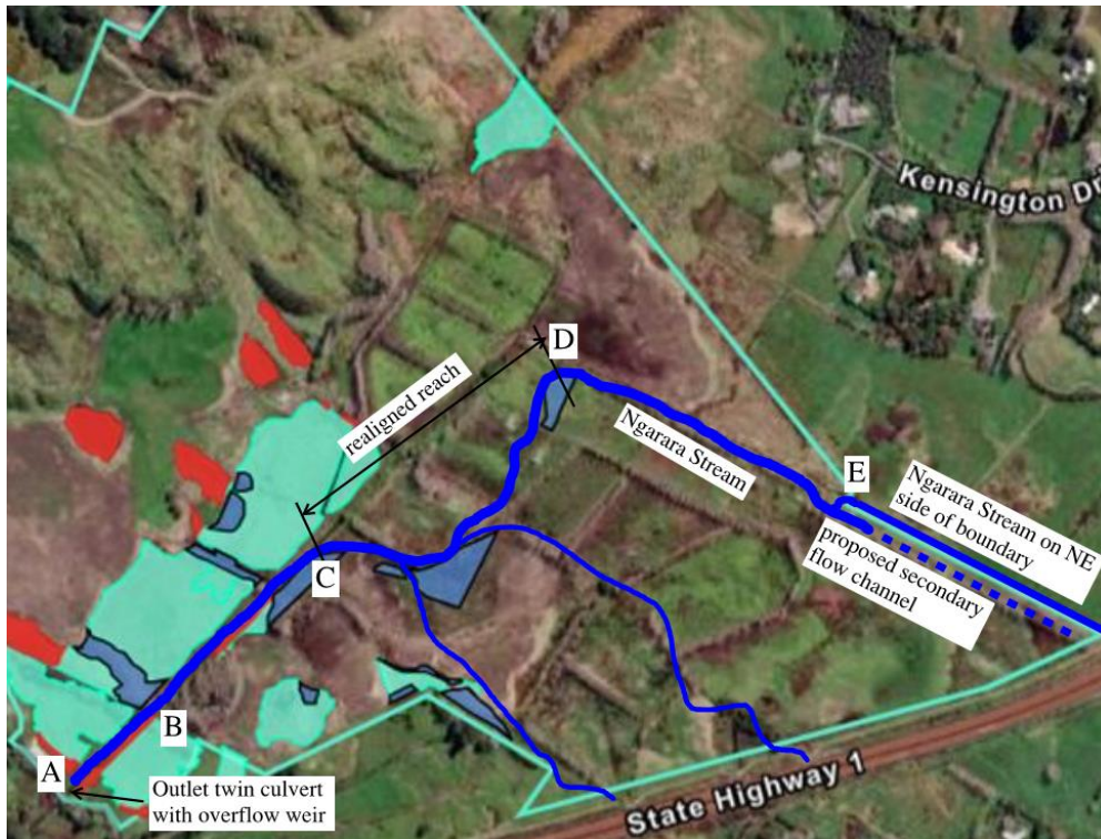
Figure 16 Ngarara Stream Realignment
