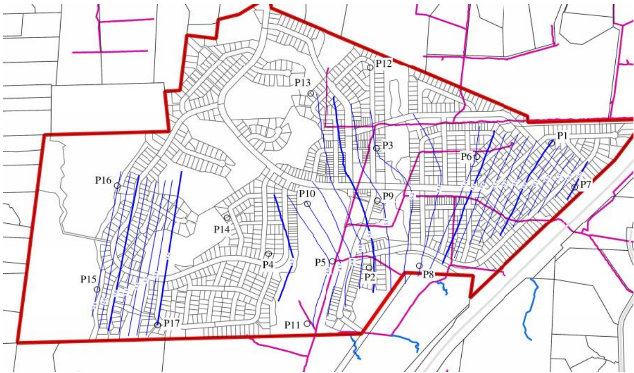
Figure 7 Groundwater Monitoring Piezometer Locations and inferred groundwater level contours
