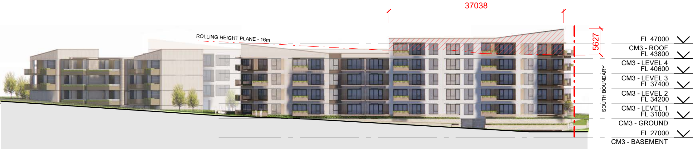
2 | 1 : 500 | Elevation CM3 - NORTH WEST STREET ELEVATION
