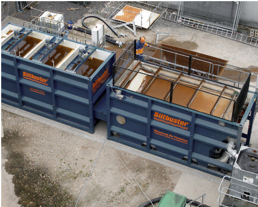
Figure 9 - Example containerised sediment control treatment unit
