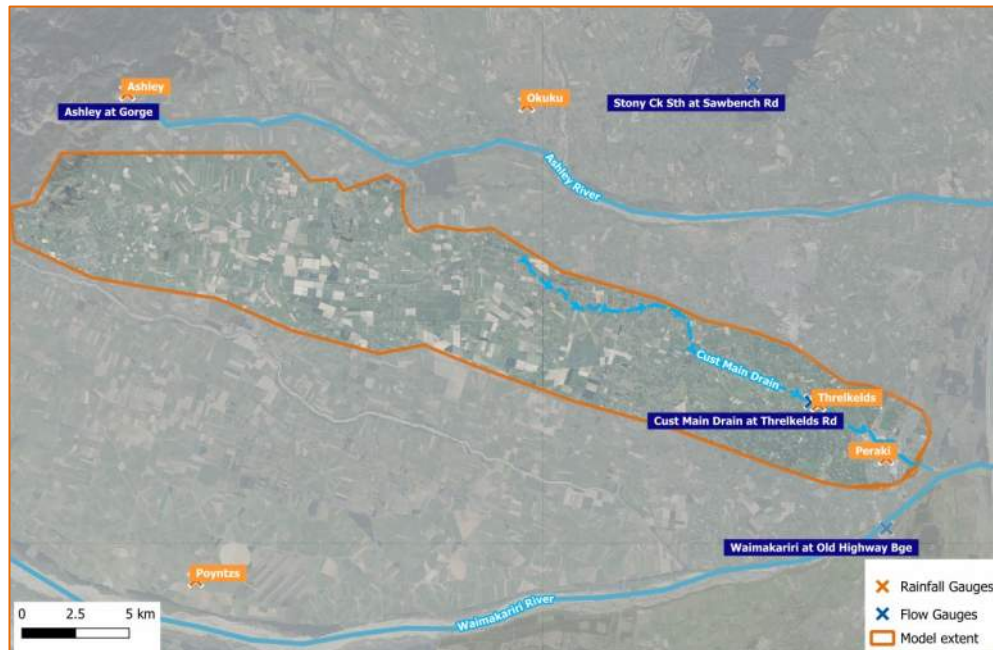
Figure 10: Flow and Rainfall Gauge Locations
