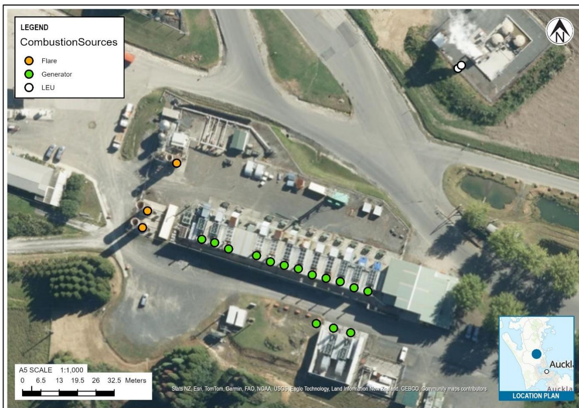
Figure 4.4: Location of discharge stacks associated with the generators, flares, and LEU
