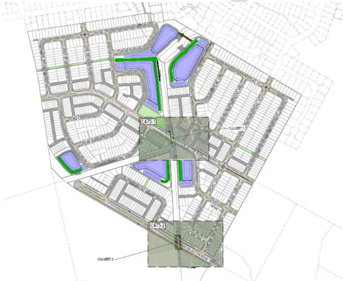
Figure 3: Proposed culvert crossing locations.
