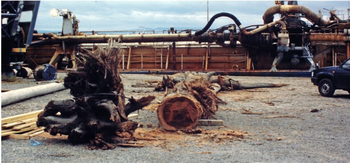
Figure 9: Examples of the larger clasts encountered by the trailer suction dredge during the 1991/92 Capital Dredging Programme: top left – shells cemented in estuarine mud; top right – wood, pumice, peat, iron cemented sands (ferricrete or iron pan) and rhyolite cobbles; and bottom – tree stumps.
