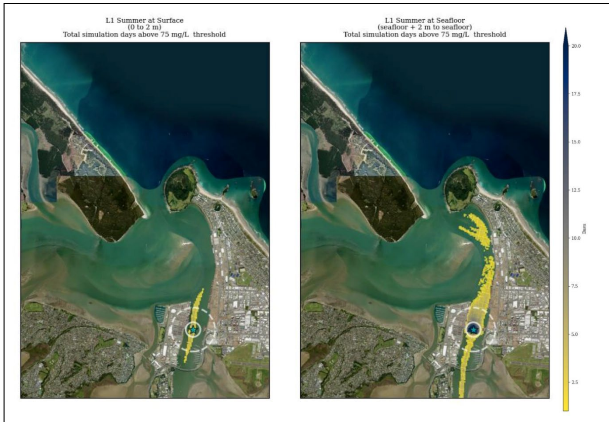
Figure 17: Number of days that peak TSS exceeded 75 \text{ mg.l}^{-1} for a large TSHD excavating sediment from the southern Stella Passage for a 65 day period. The surface plume represents the surface 2 m of the flow, and the seafloor plume represents the deepest 2 m. The point of release is marked by a star, and surrounding circles represent a 200 m (solid line) and a 600 m (dashed line) circumference to identify the mixing zone. (Figure 3.5 from Montaña, 2024).
