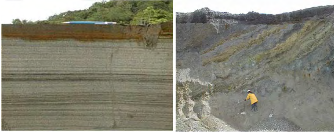
Figure 7. Diffusion of oxygen into a TSF as shown by Fe oxidation products, and advection pathways within a WRD as shown by oxidation at angle of response tipheads.
