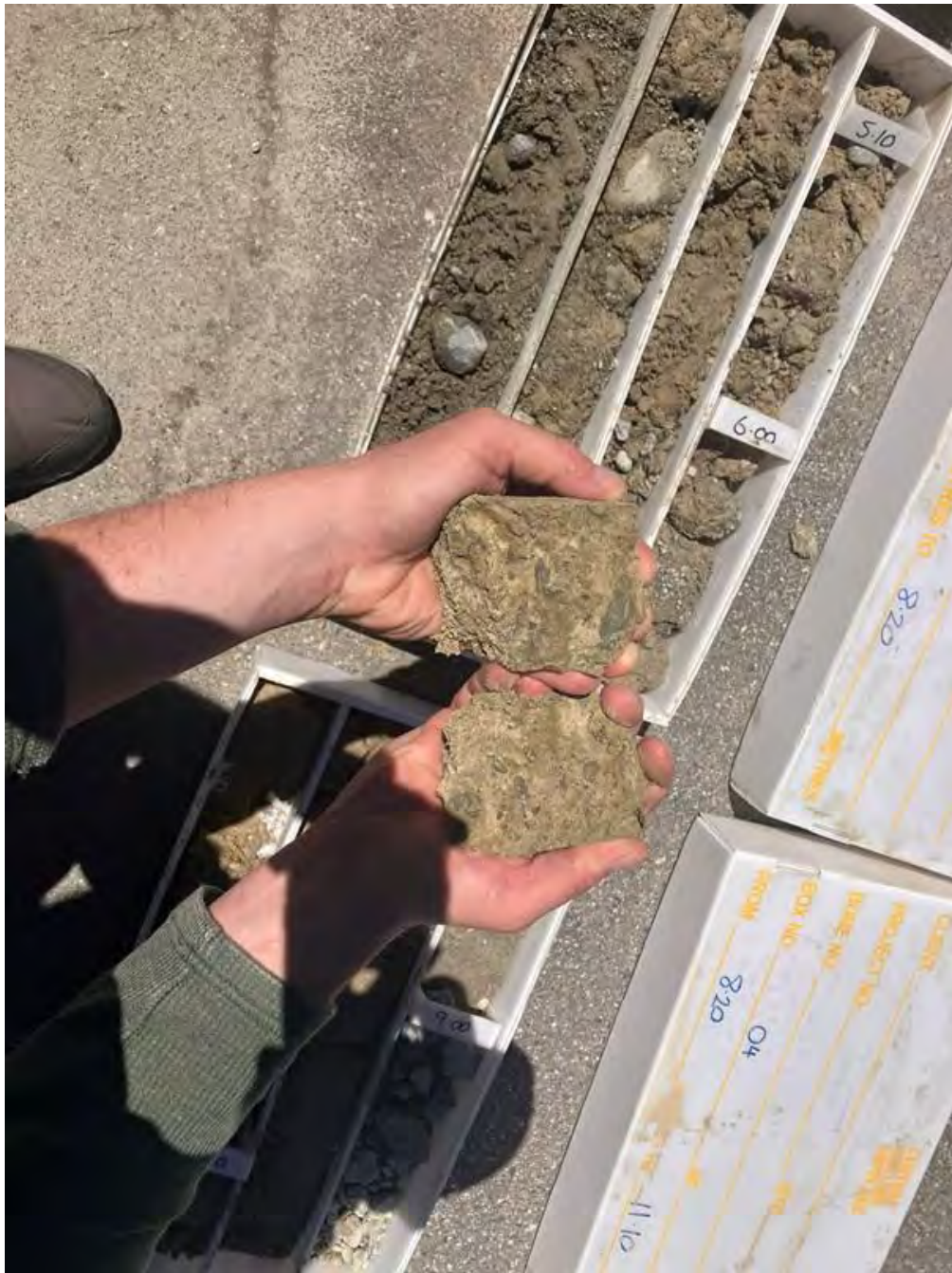
Photograph 4B - Drill core at 10.8 m depth, Glacial Till
