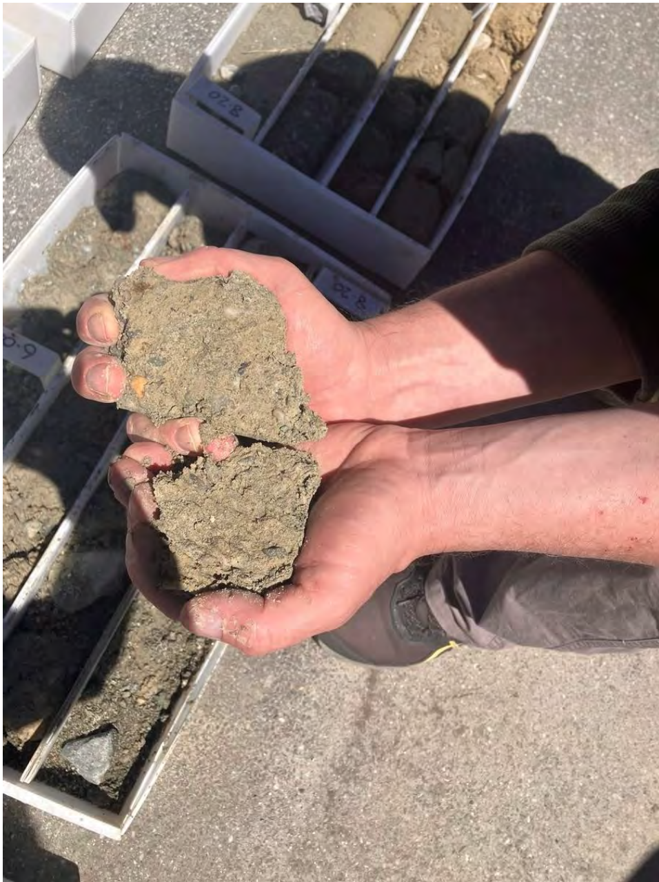
Photograph 3B - Drill core at 6.0 m depth, Glacial Till like, suggesting transitional depositional process of alluvial fan, glacial outwash and re-working glacial till and reworked deposits.
