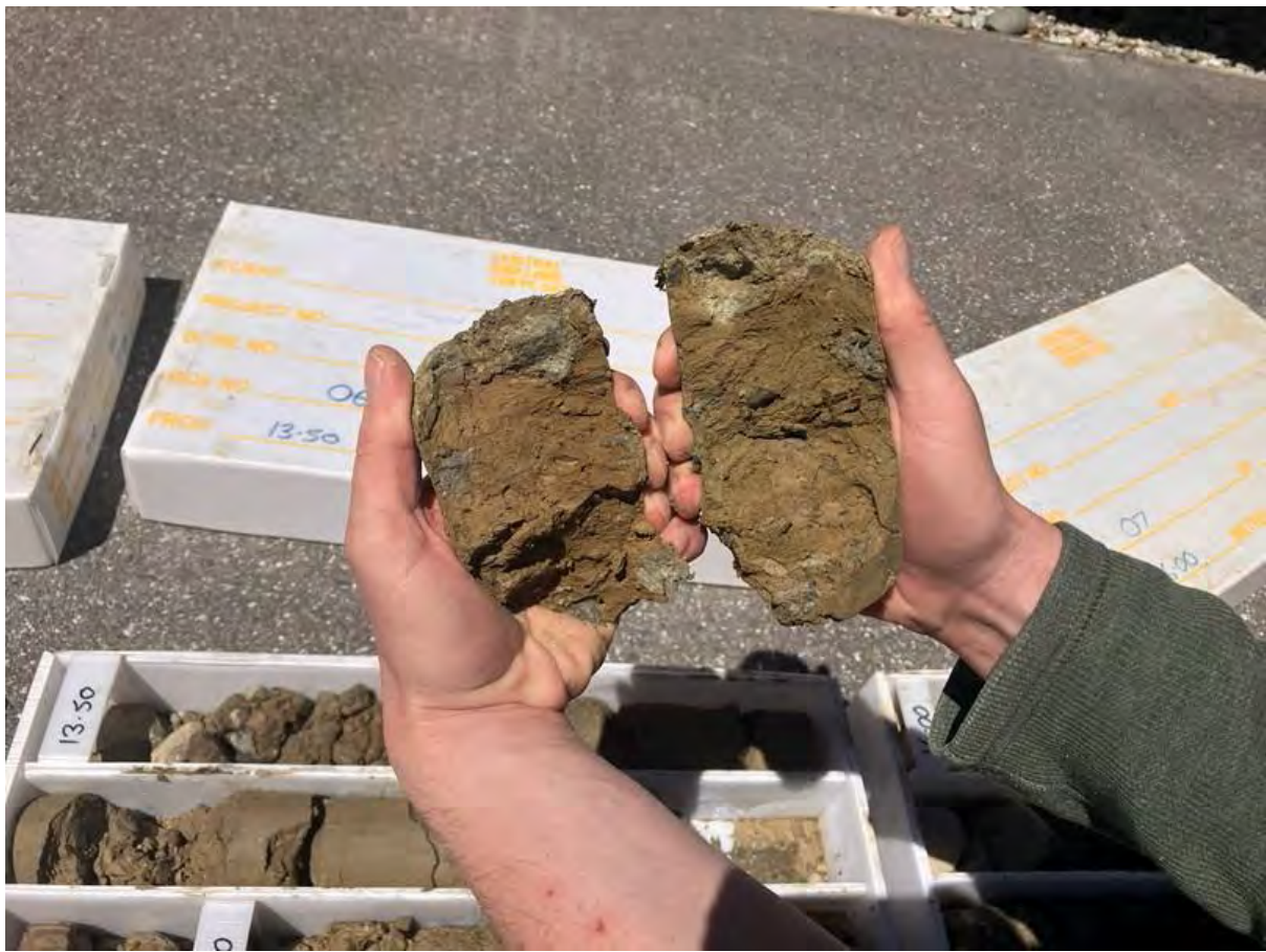
Photograph 5B: Drill core at approximately 14 m depth, Glacial Till.
