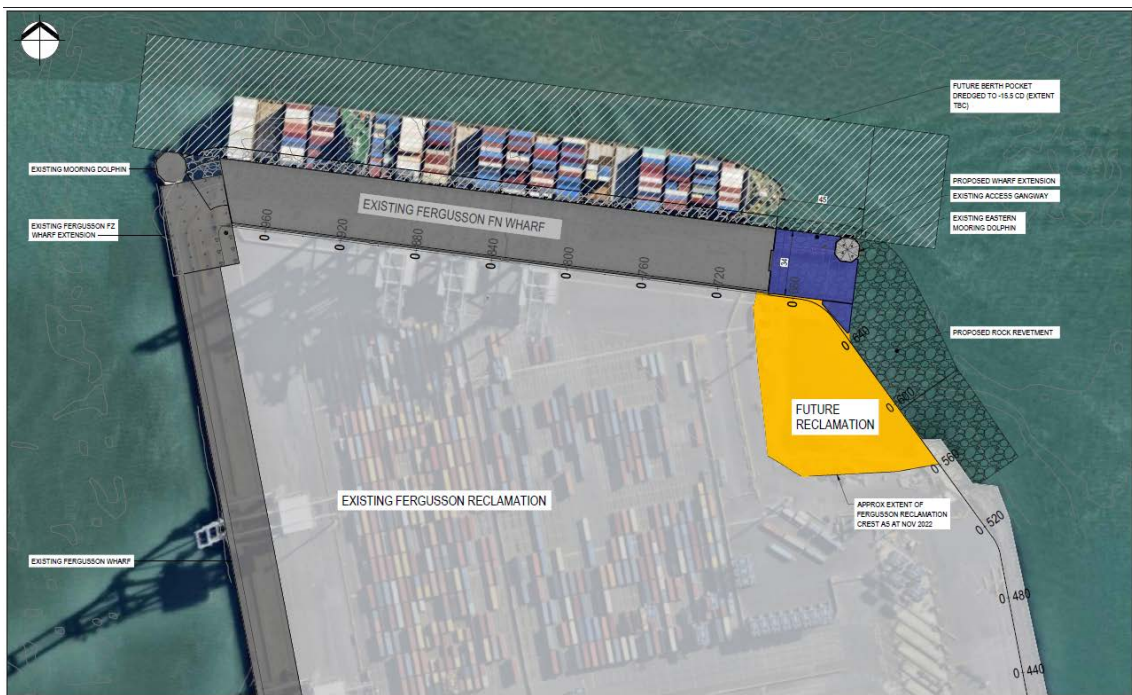
Figure 4: Proposed Fergusson North Wharf Eastern Extension (blue) and already approved future reclamation (in yellow), and proposed Revetment (circular hatch) which is part of the already consented reclamation)
