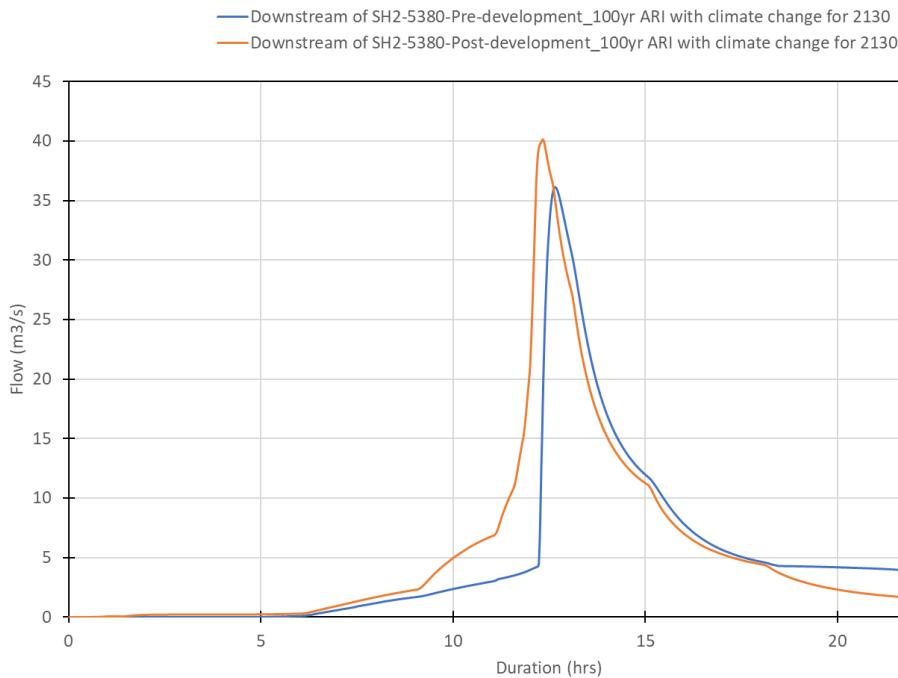
The peak flows downstream of culvert SH2-5180 and bridge SH2-5380 are higher in post-development condition as compared to pre-development condition which is primarily due to replacing of the existing culvert at Oturu Creek Tributary with a new culvert named SH2-5180 and replacing of the existing culvert at Oturu Creek with a new bridge named SH2-5380.
