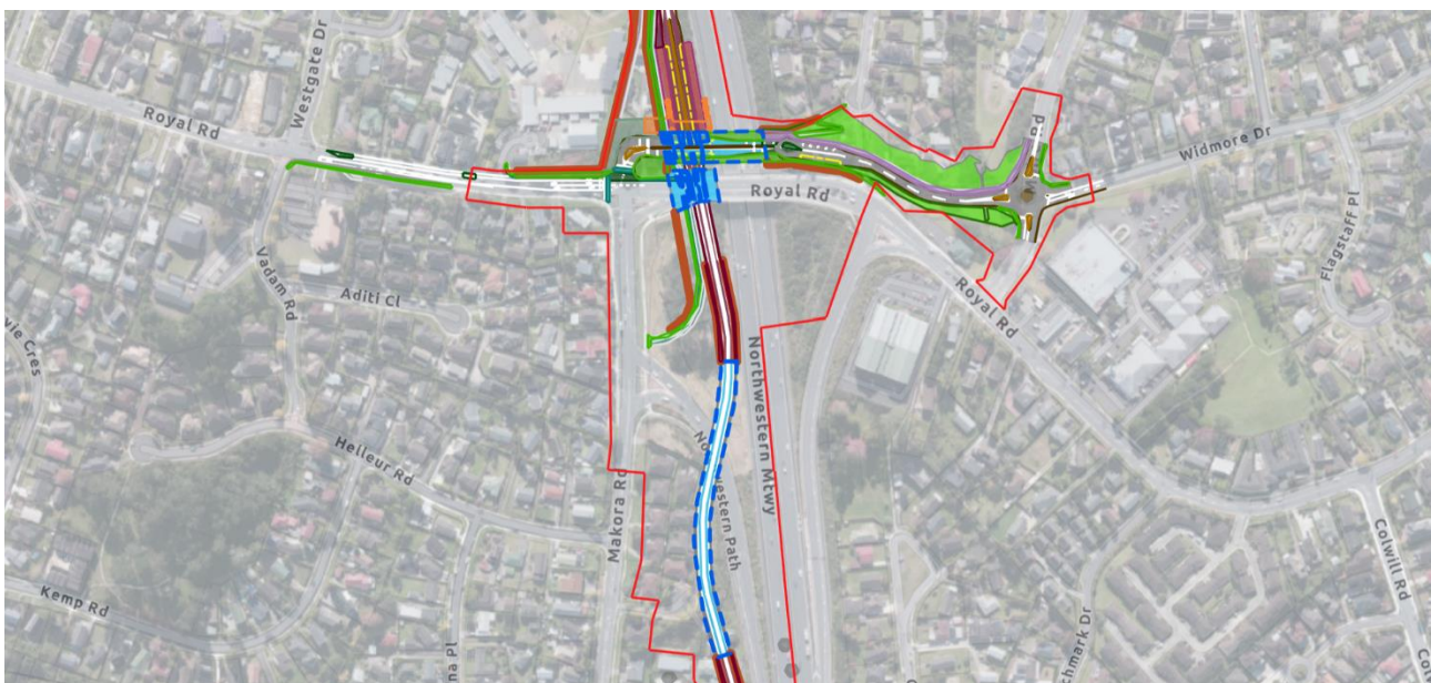
Figure 4-3: Plan of the Royal Road station location, busway carriageway, underpass, new bridge over SH16 and the Makora Road viaduct bridge
