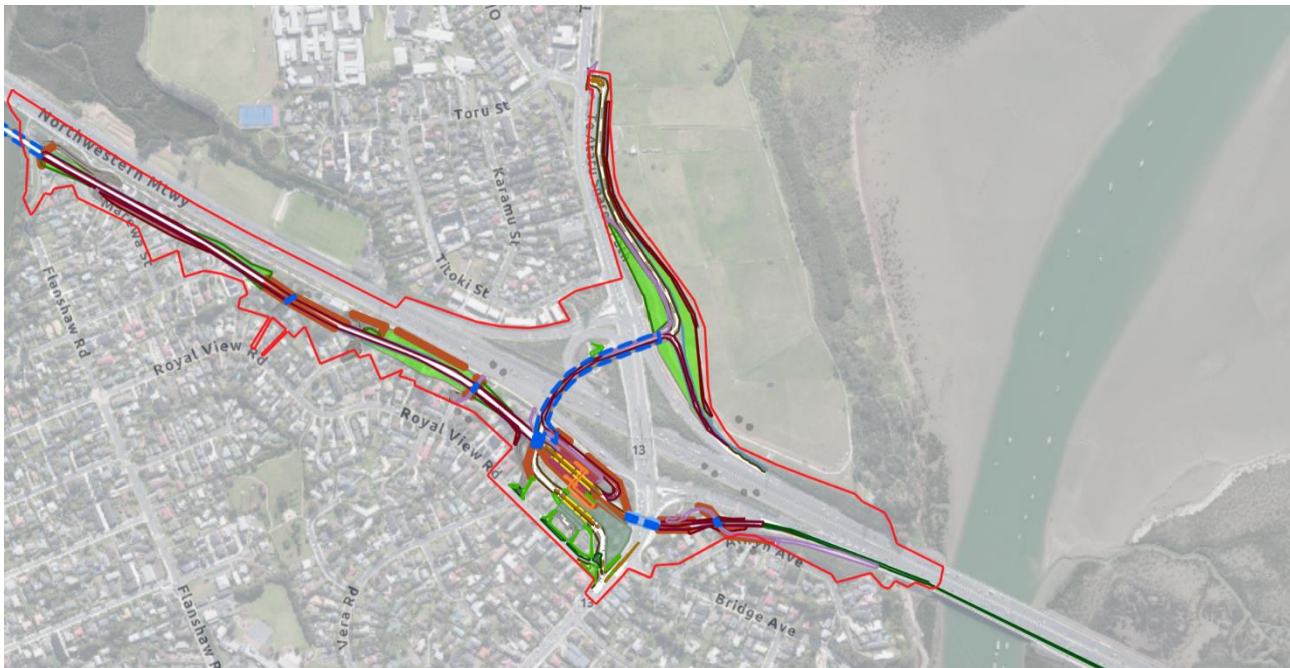
Figure 4-5: Plan of the Te Atatū station location, proposed new bridge over SH16 and the extent of the Proposed Designation
