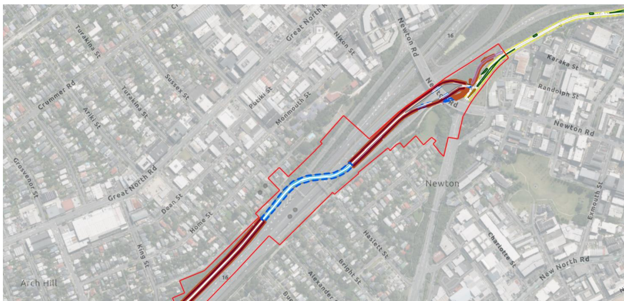
Figure 4-8: Plan of the new bridge (blue) over SH16 which connects through to Ian McKinnon Drive in the context of the existing infrastructure and elements in the localised context
