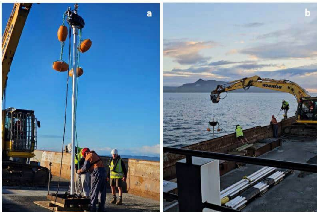
Figure 2.3: A) Preparation of the vibracore for seafloor drilling, note the 5 m aluminium barrel (rod) attached to the vibracore rig and drilling frame. B) A 23 T excavator winching the vibracore rig to the seafloor for drilling operation.
