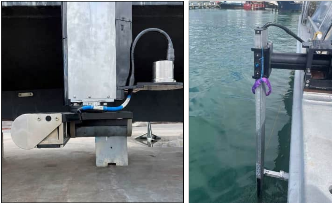
Figure 4: MBES Sonar and Motion unit (left) and over the side mount (right)
