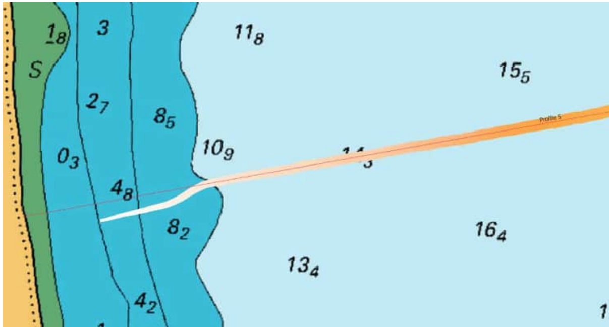
Figure 9: showing deviation from profile line due to fisherman
