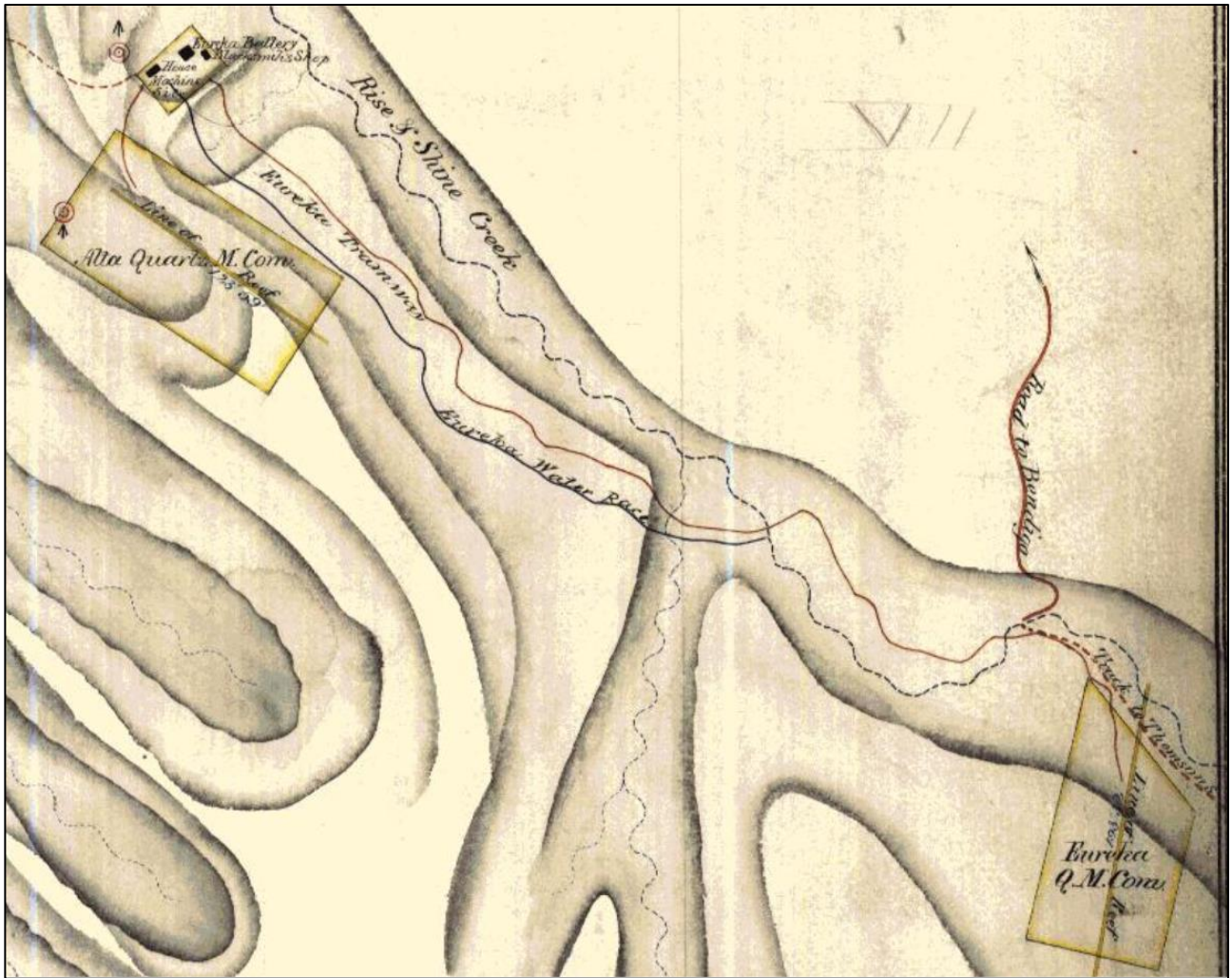
Figure 5 Survey plan SO 2086 (1876) showing the Eureka reef at the location of the Rise and Shine mine and battery site (G41/277), in relation to the Eureka mine and battery site (G41/252) and the Alta reef around the site of the Alta battery site (G41/253). The plan also shows the Eureka Water Race and the Eureka Tramway recorded as part of the Eureka Mine and battery (G41/252) (Source: QuickMaps).
