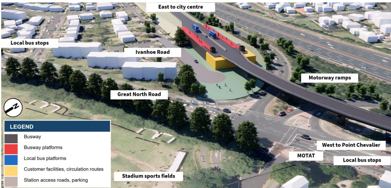
Figure 1-11: Western Springs station indicative design
