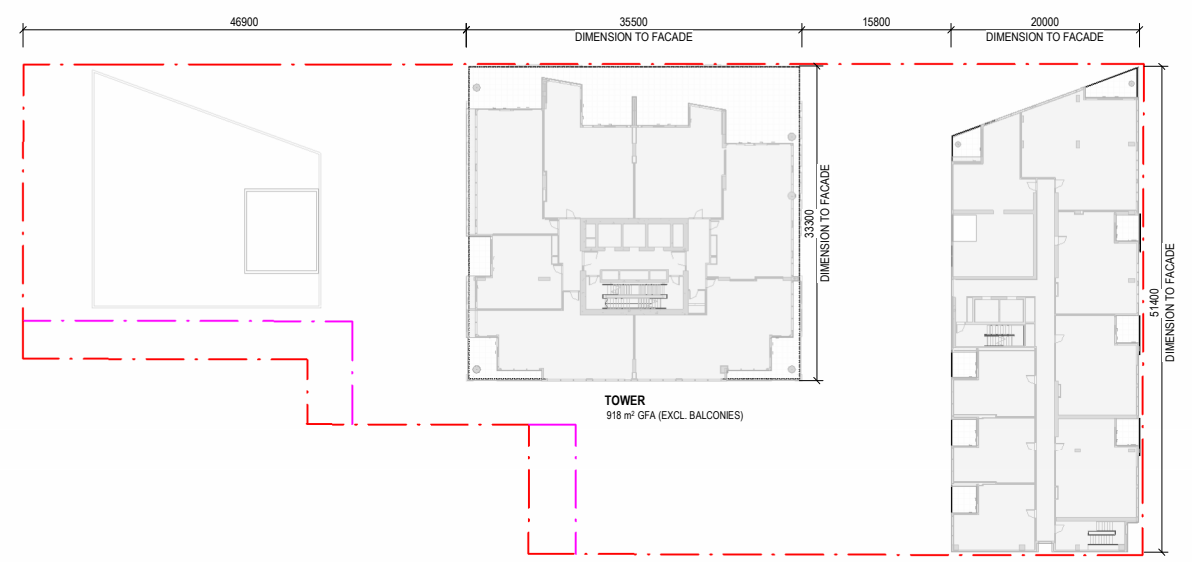
BUILDING FLOOR PLATE DIMENSIONS ABOVE 31m - LEVEL 9
