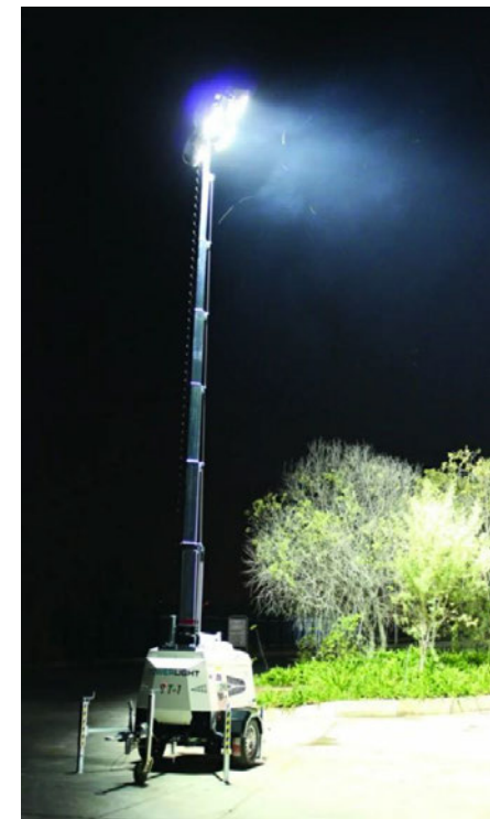
Figure 10: Typical Mobile Lighting Plant
