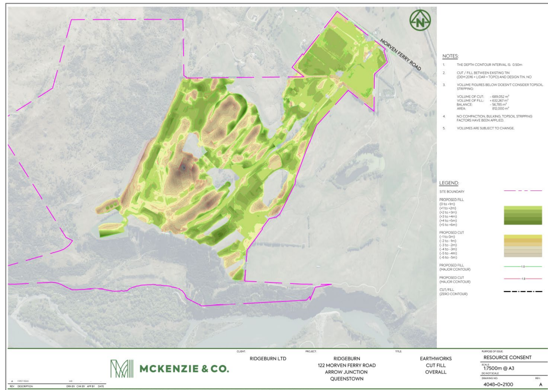
Figure 62: Ridgeburn bulk earthworks cut and fill plan.
