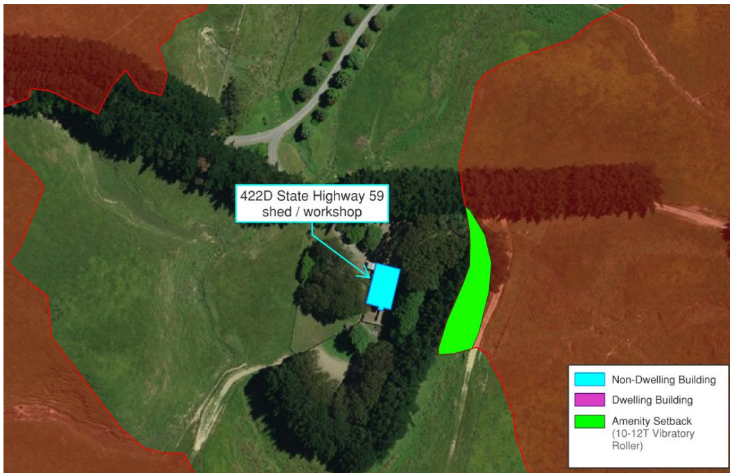
Figure 1: Vibration amenity setback within Earthworks footprint for 422D SH59 (10-12T vibratory roller)
