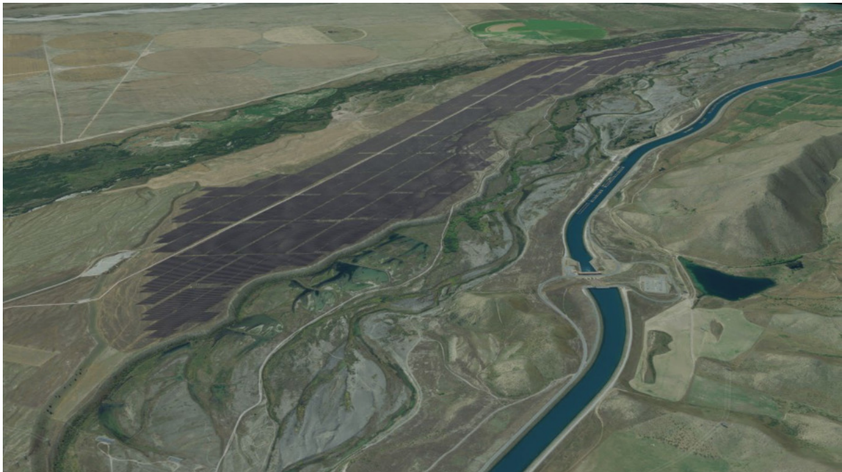
Overview of the 3D model, showing the digital terrain model with the solar panel layout.
