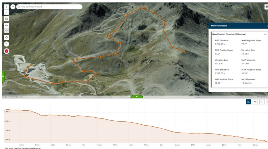
Figure 14. Option 2 layout and long section showing localised low and high points
