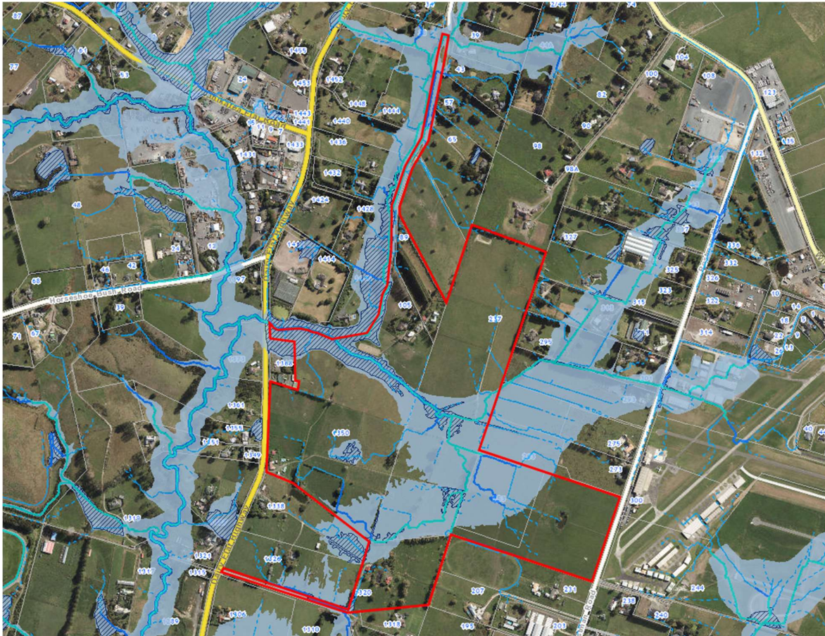
Figure 6 - Existing OLFP (dark/light blue solid and dashed lines), Streams (cyan lines), Flood Prone Area (dashed blue area) and Floodplain (sky blue area). (Source: Geomaps, 2025)
