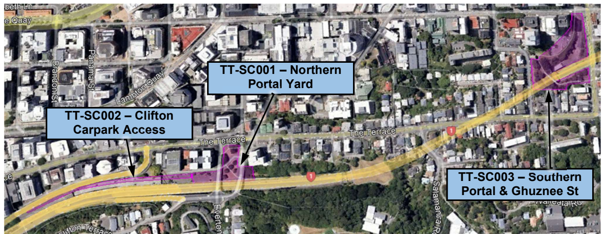
Figure 2 - Construction yards/laydown identified around the Terrace Tunnel
