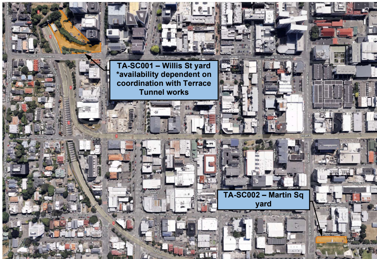
Figure 3: Construction yards/laydown in Te Aro
