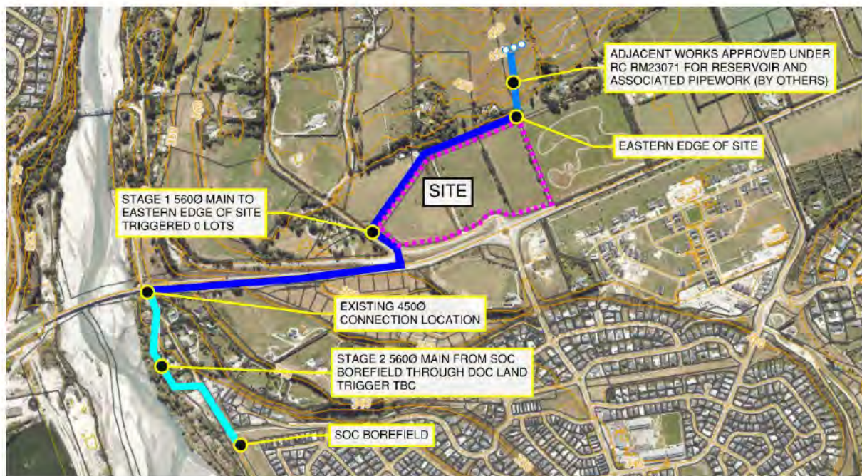
Figure 11 – Proposed External Water Infrastructure
