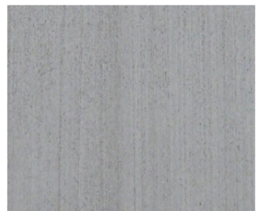
Joal Mix 2 (Carriageway and Joal Footpath) Broom finish concrete with 5kg/m³ black oxide
