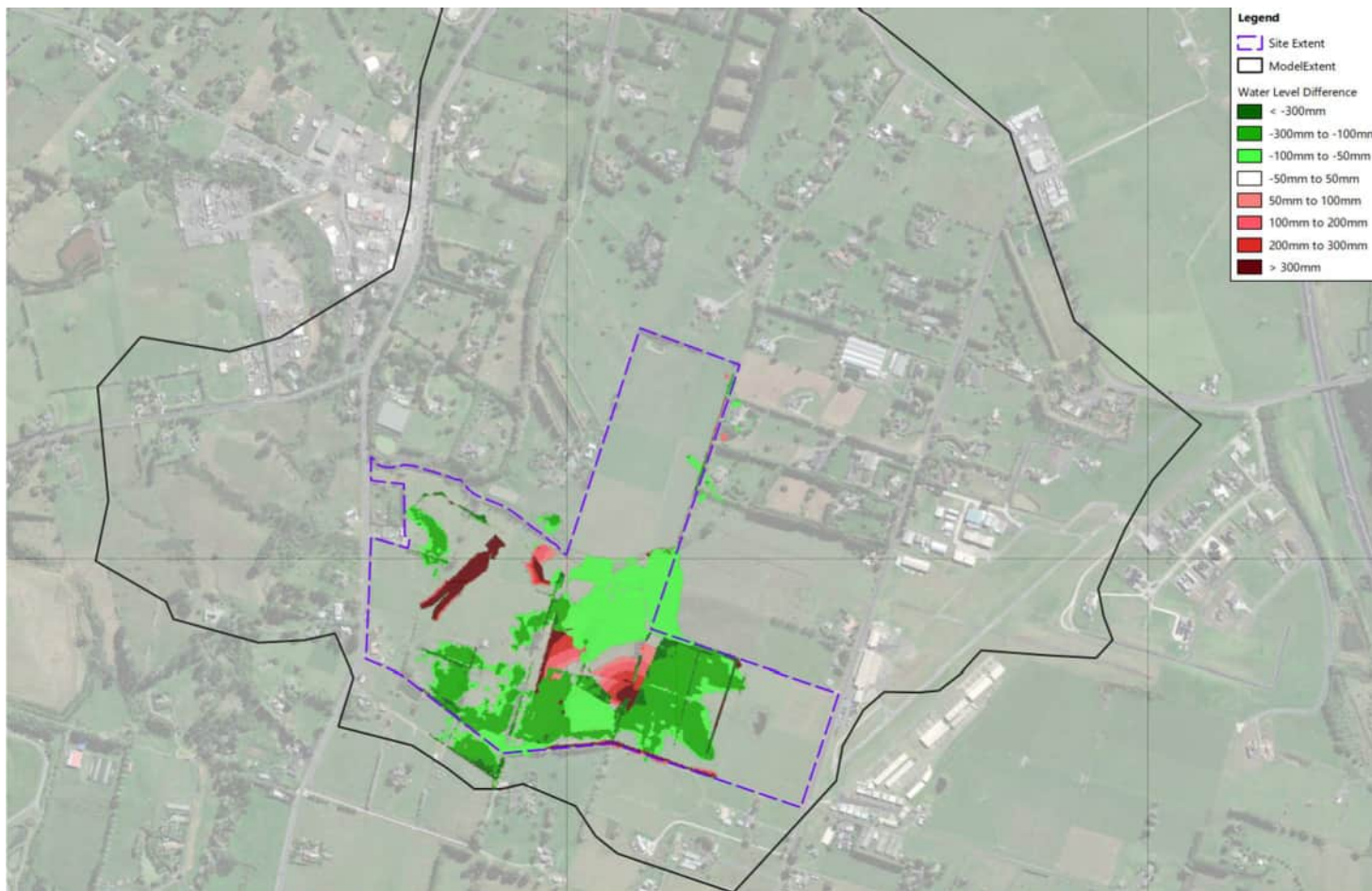
Figure 9: Water level difference – Scenario 2 vs Scenario 1 100-year ARI 3.8°C CC
