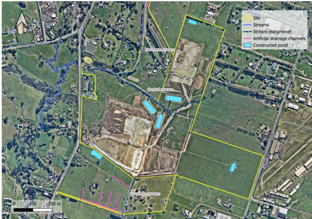
Figure 9. Freshwater features within the site.
