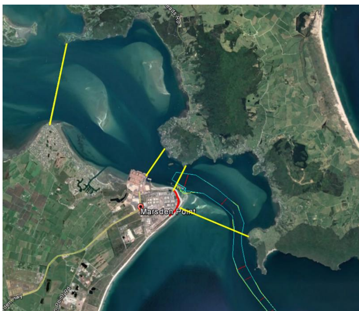
Figure 3-20: Location of transects (yellow lines) to calculate tidal flux
