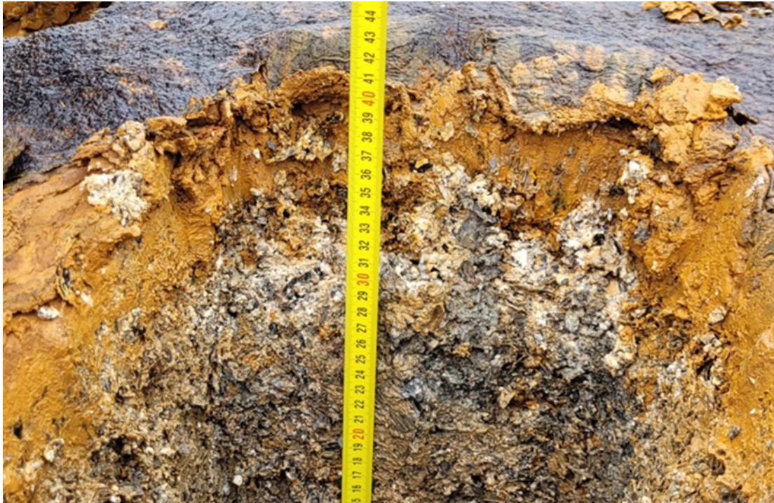
Figure 18: Sludge and Fe + Al precipitation zones within the BV-MSR.
