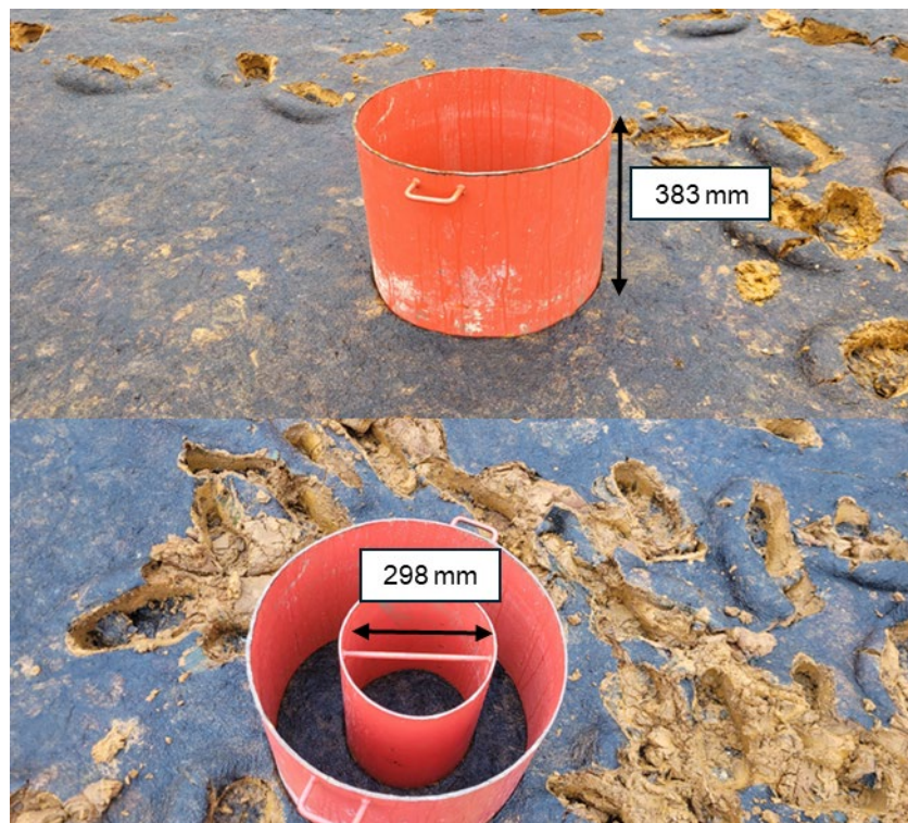
Figure 12: Infiltrimeter on BV-MSR sludge layer.
