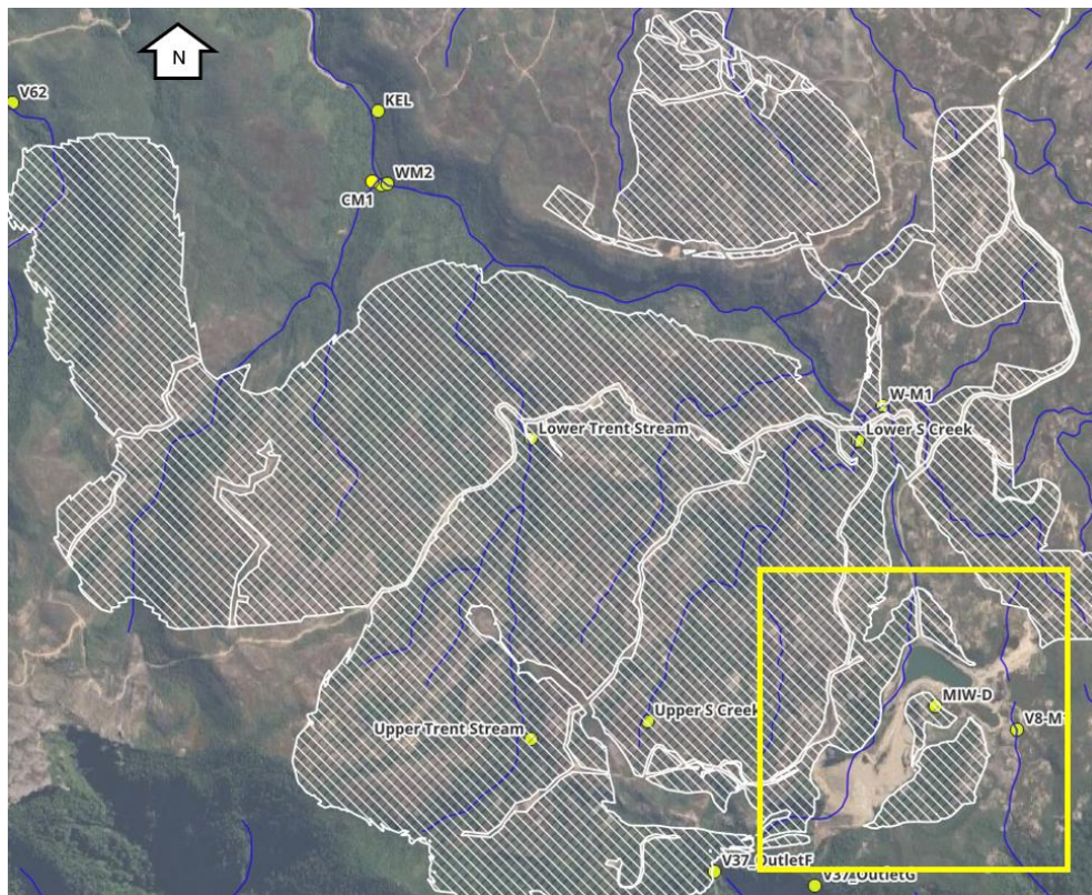
Figure 37: Detail of Escarpment Extended mine area (white hatched) which drains north to the Whareatea River and south to Cascade Creek
