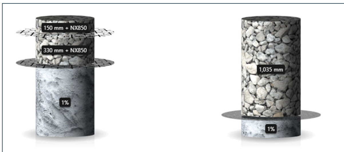
Figure 19: Unreinforced pavement structure and tensar reinforced pavement structure
