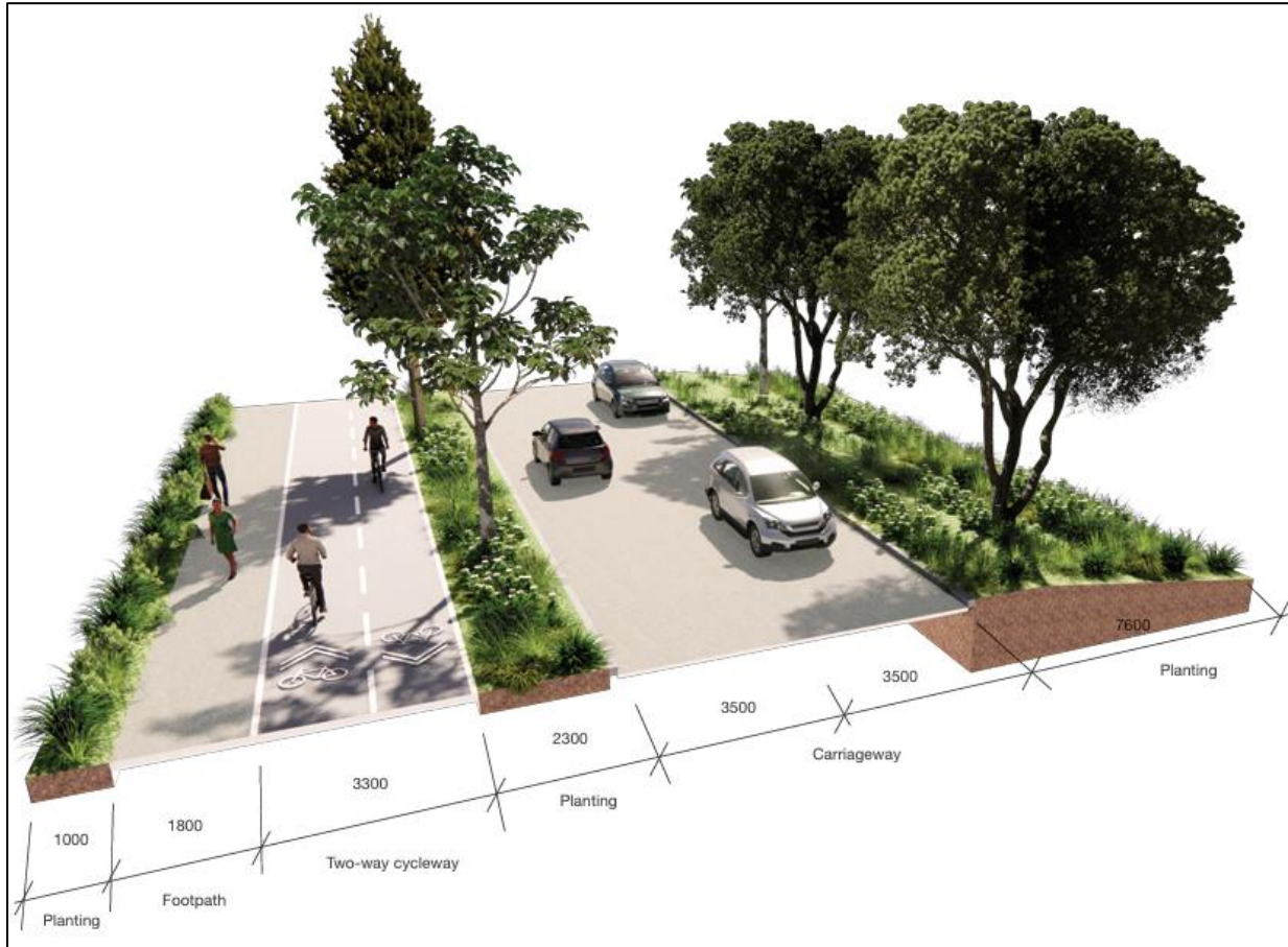
Figure 7-17: Proposed Jack Lachlan Drive Cross Section (Segment B - Between Boat Houses and Kahawairahi Drive)
