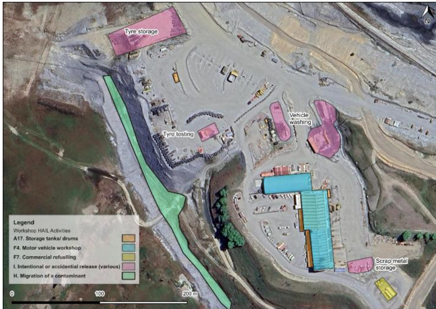
Figure 6-18: Existing Workshop Layout (Source: WWLA, 2026b).
