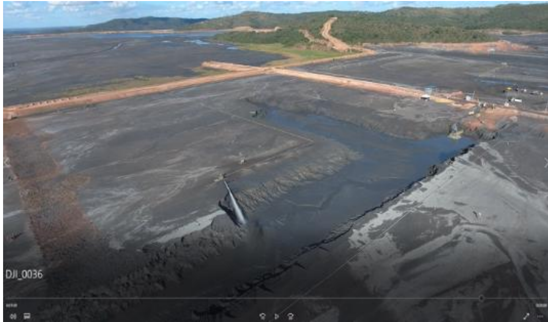
Figure 6-16: Bench and Mining Block Development during Hydraulic Mining
