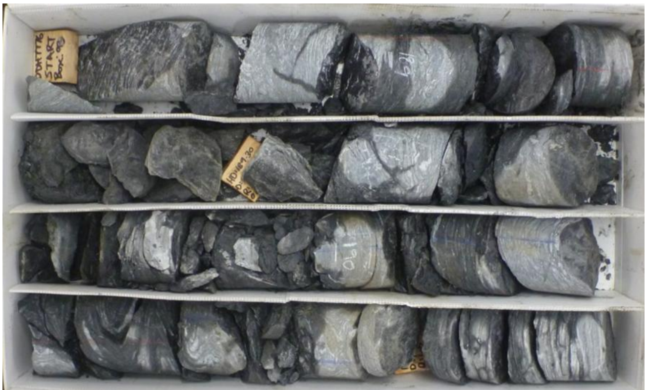
Inset 12: Fractured Zone – Example from DDH7776.
