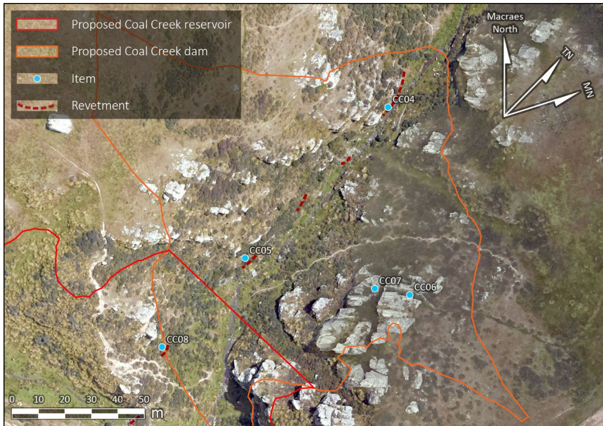
Figure 152. Features recorded in the proposed dam footprint; red dashed lines indicate revetments (2025 OGNZL aerial photography).
