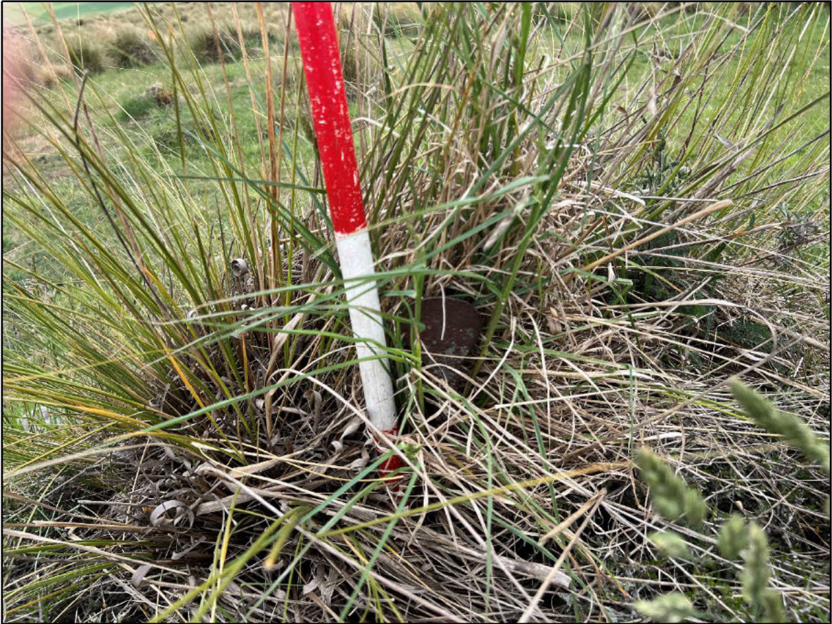
Figure 139. Bayonet type survey marker at Trig D.
