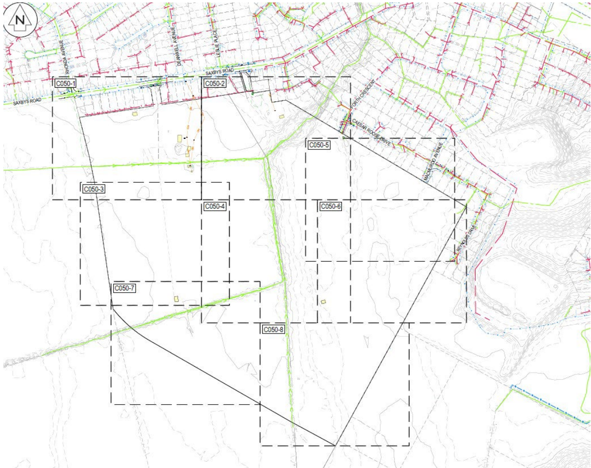
Figure 4: Existing Site Stormwater Layout
