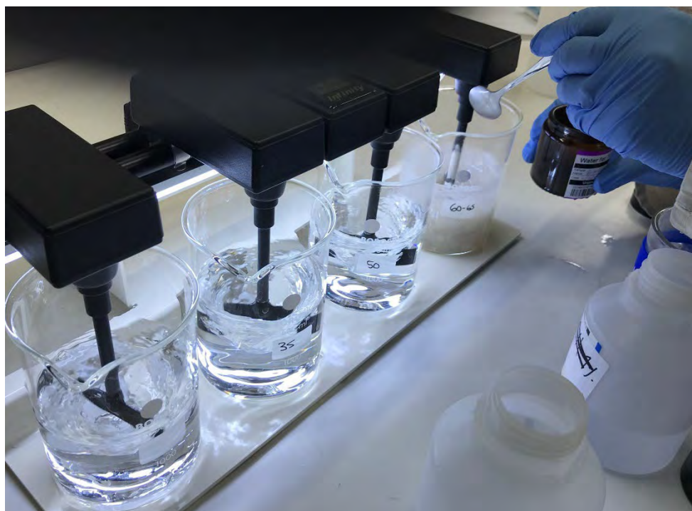
Figure 2 Farmguard Start of Slaking Process, makeup water at 20, 35, 50 and 65°C in jars left to right respectively.
