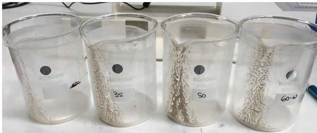
Figure 9 EMag45 residue after slurry removed from jars
