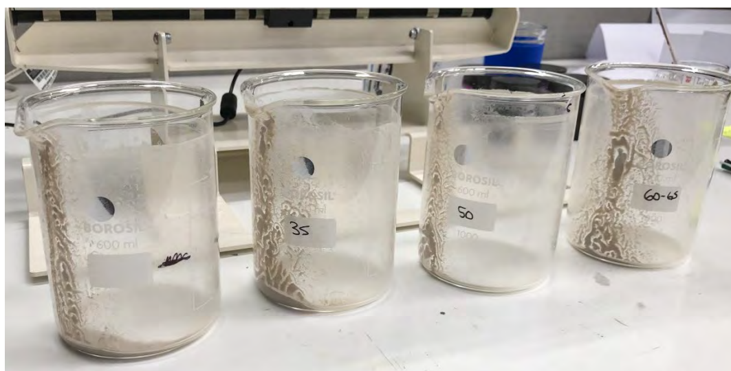
Figure 9 EMag45 residue after slurry removed from jars
