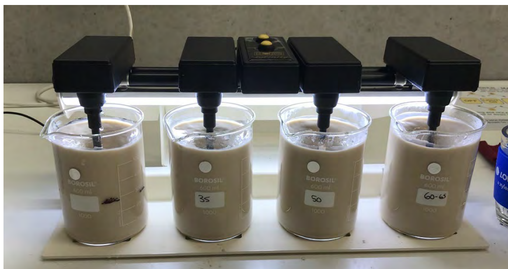
Figure 2 Farmguard Start of Slaking Process, makeup water at 20, 35, 50 and 65°C in jars left to right respectively.
