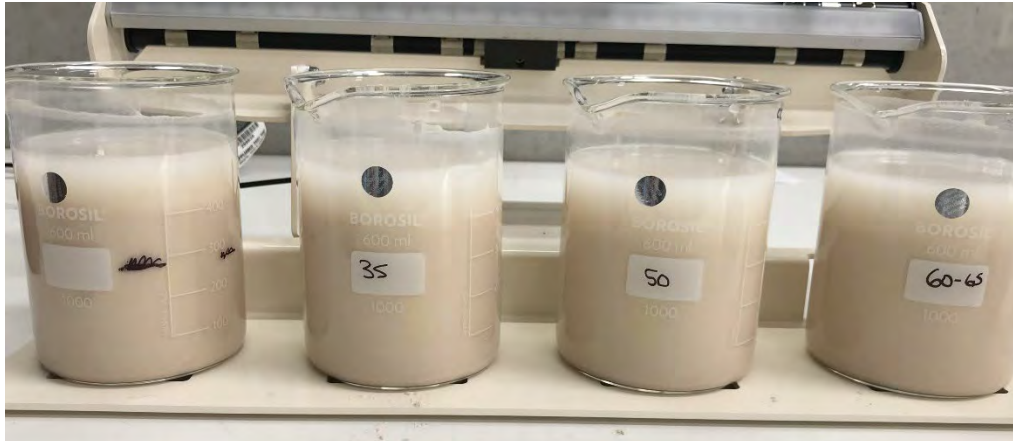
Figure 6 Farmguard Slurry 2 minutes after slaking finished, already settling out.
