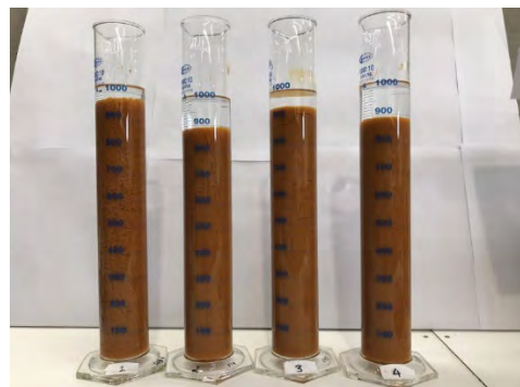
Figure 8 Sludge Thickening - S23 with Rheomax 1030
