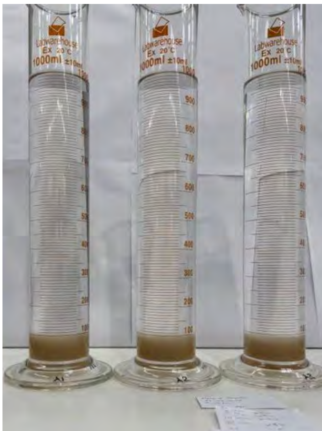
Figure 4 Makeup Water Testing - 30 mins settling
