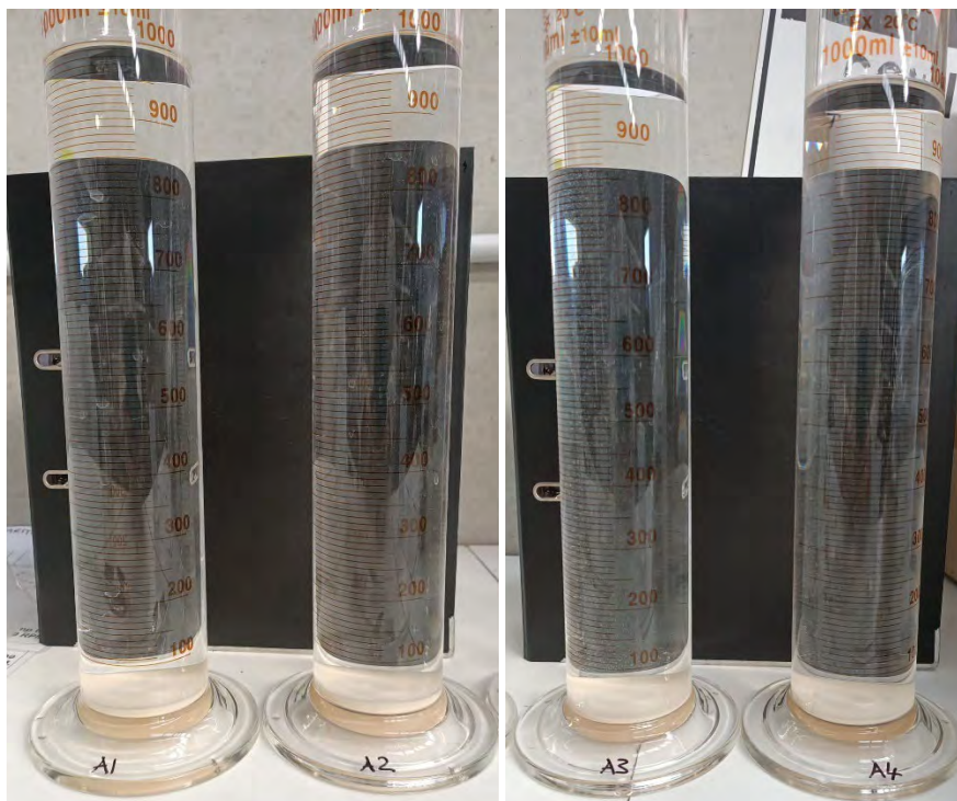
Figure 13 Neutralisation, Coagulation, Flocculation and 24 hours Settling - samples Farm 20°C, Farm 55°C, Emag20°C and Emag 65°C left to right.
