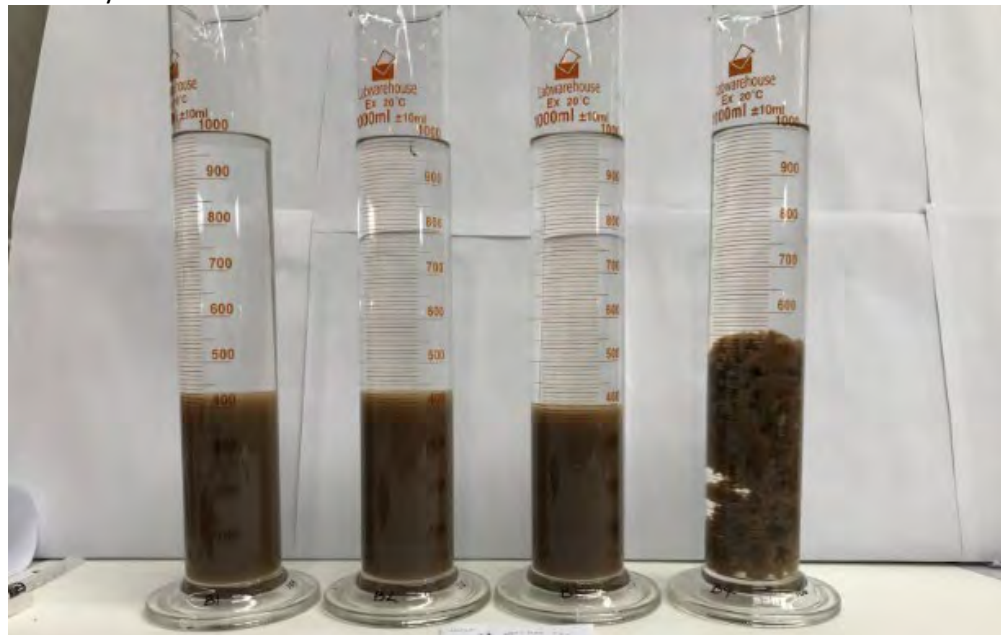
Figure 7 Sludge Thickening - S23 with Rheomax 1050
