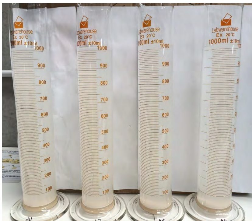
Figure 12 Neutralisation, Coagulation, Flocculation and 30 minutes Settling - samples Farm 20°C, Farm 55°C, Emag20°C and Emag 65°C left to right.
