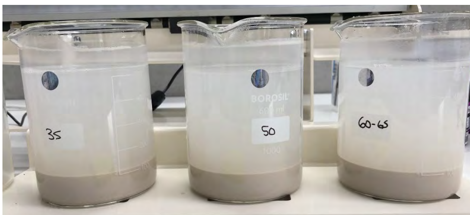
Figure 7 Emag45 slurry 2 minutes after slaking, settling rapidly in jar - not suspended
