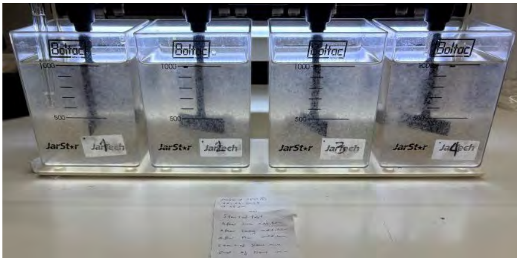
Figure 2 Floc Formation at end of Slow Mix - Makeup Water Testing
