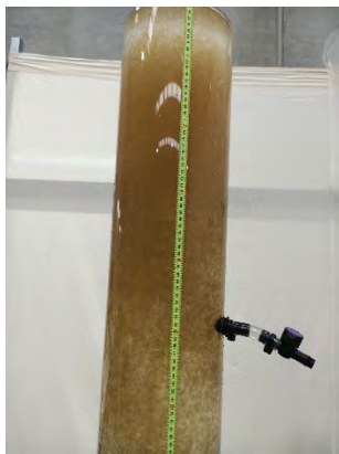
Figure 3 Column Settler showing Floc reformation after water transfer
