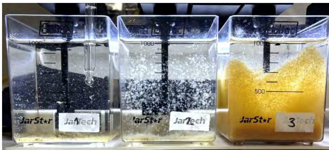
Figure 4 Barren Valley ELF, Manchester St and S23 AMD at Slow stir Flocculation stage
