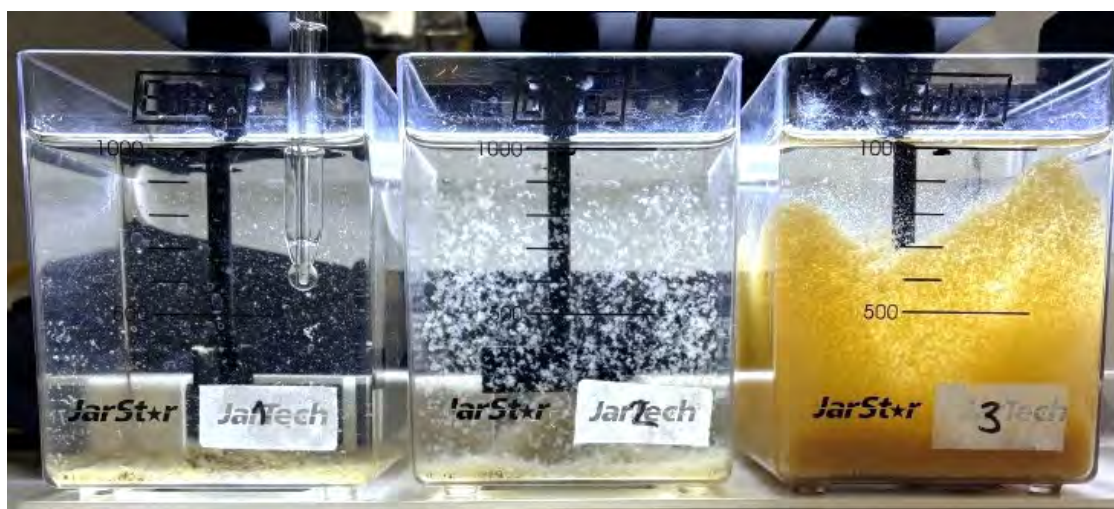
Figure 16 Barren Valley ELF, Manchester St and S23 AMD at Slow stir Flocculation stage
