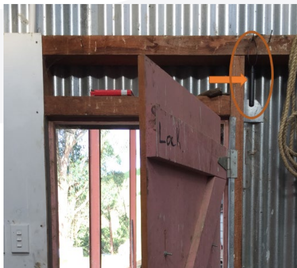
Photo 16: Baro logger hanging on nail inside locked shed (that houses the ATV).
