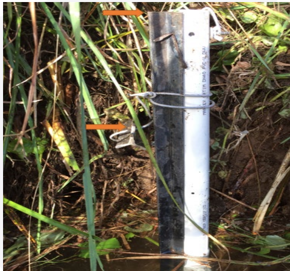
Photo 11: Logger housed in plastic pipe attached to waratah. Level taken from top of logger waratah and top of lateral waratah (as indicated) as distance to water surface.
