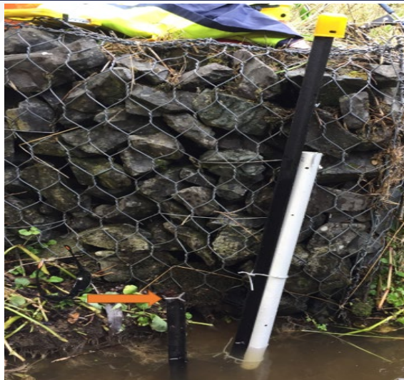
Photo 6: Logger housed in plastic pipe attached to waratah. Level taken from top of short waratah (as indicated) as distance to water surface.
