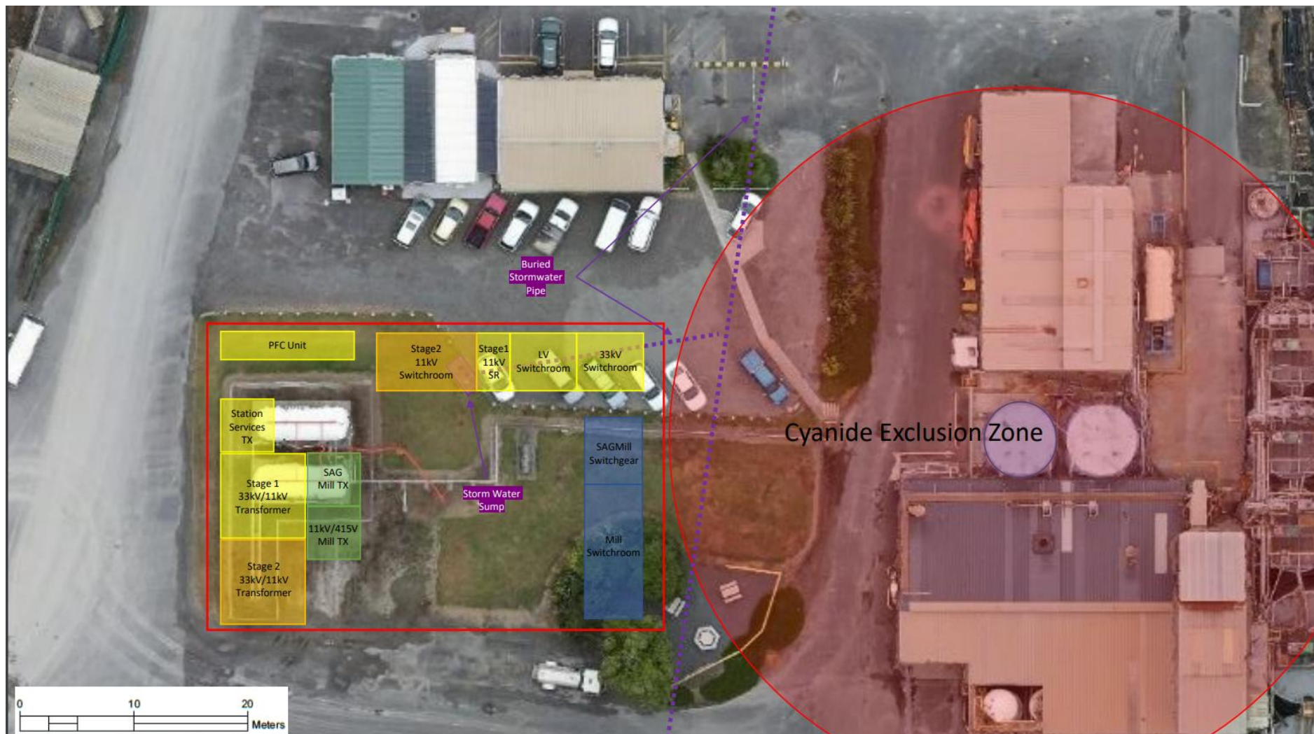
Figure 2-51: Proposed New Mine Substation
