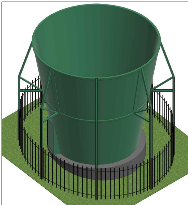
Figure 2-19: Typical Surface Ventilation Evasé
