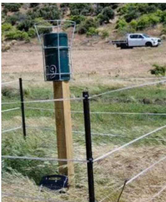
Figure 27: Photograph of the dust deposition gauge (lefthand panel) and real time dust monitoring equipment (right hand panel).
