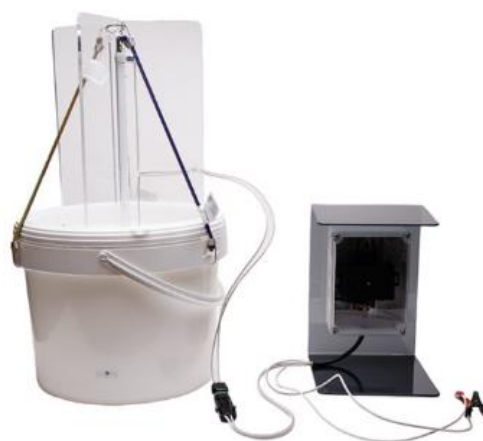
Figure 6: Light trapping equipment showing lamp and Perspex vanes secured to collection bucket and connected to automatic dusk/dawn timer
