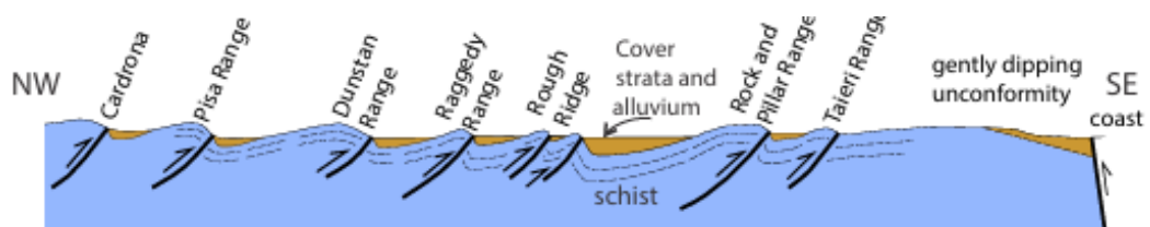
Figure 2-13: Schematic Cross-Section across the Otago Region to illustrate formation of Characteristic Basin and Range Topography. 20
