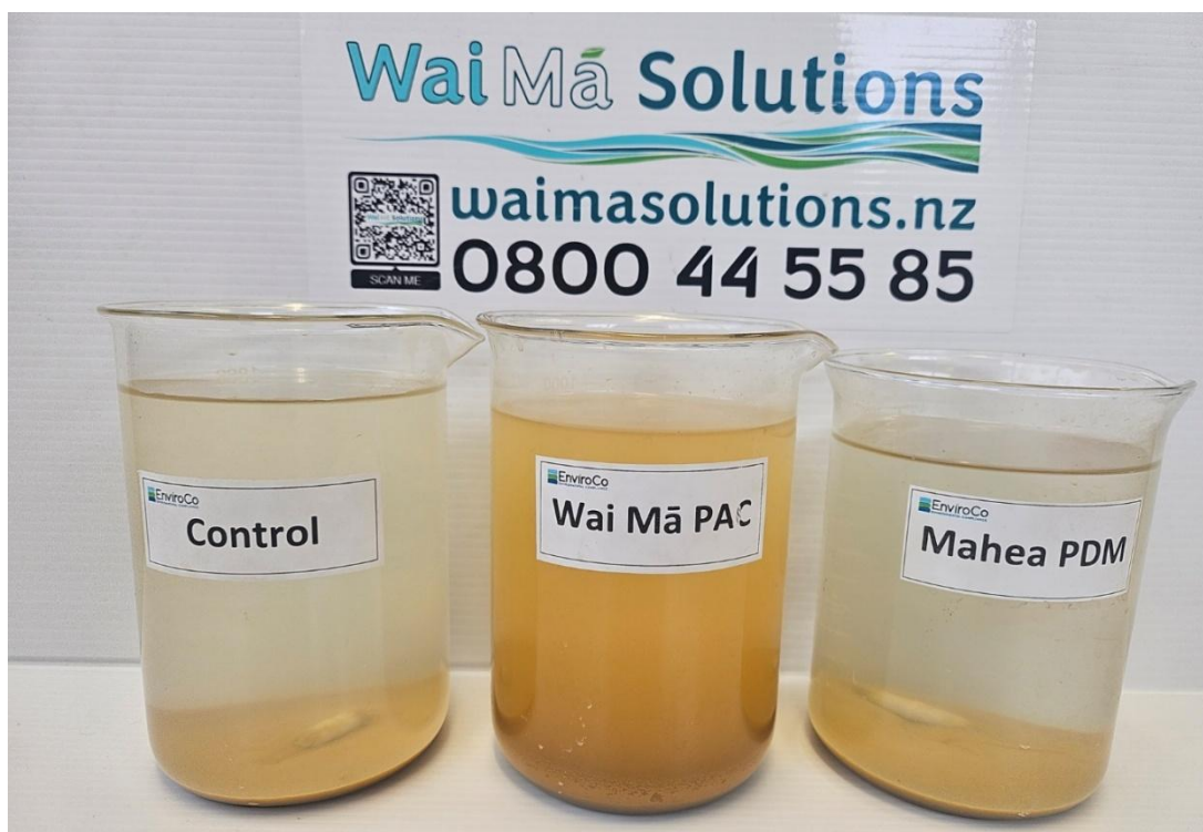
Figure 16. TPP 291 Bench testing results of liquid chemical treatment.
