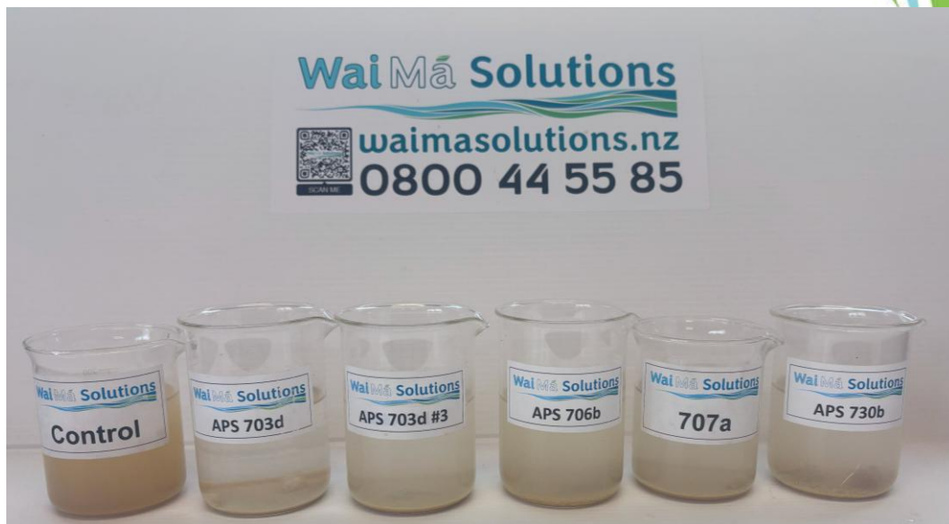
Figure 14. TPP 291 Bench testing results of Flocculants.
