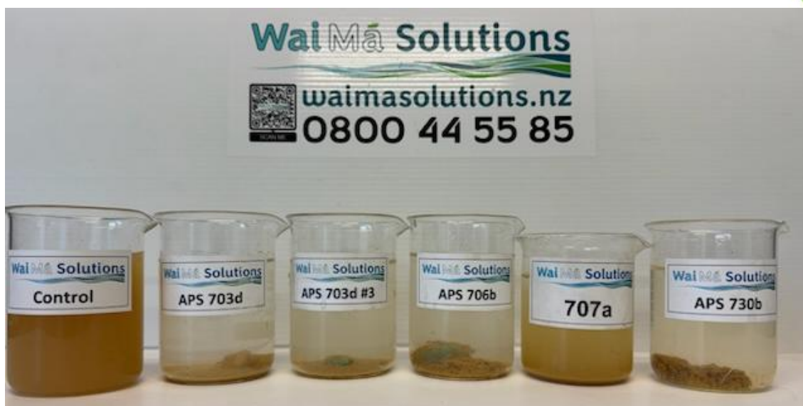
Figure 11. TPP261 Bench testing results of Flocculants.
