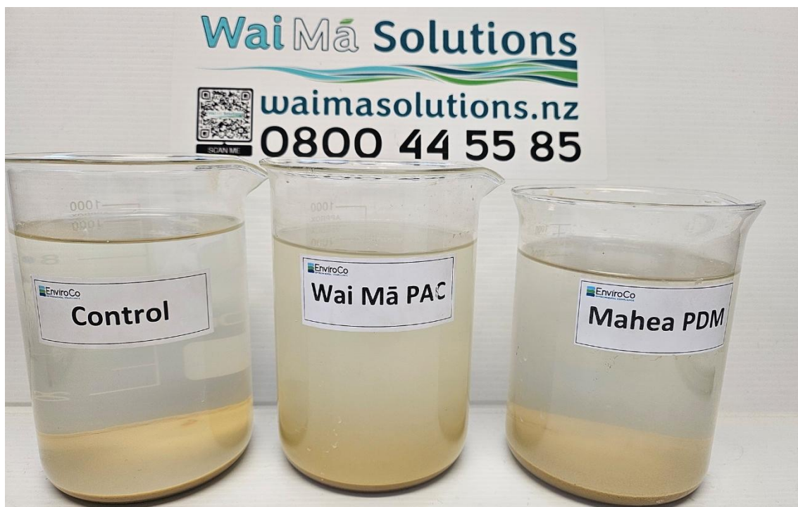
Figure 8. TP224 Bench testing results of Flocculants.
