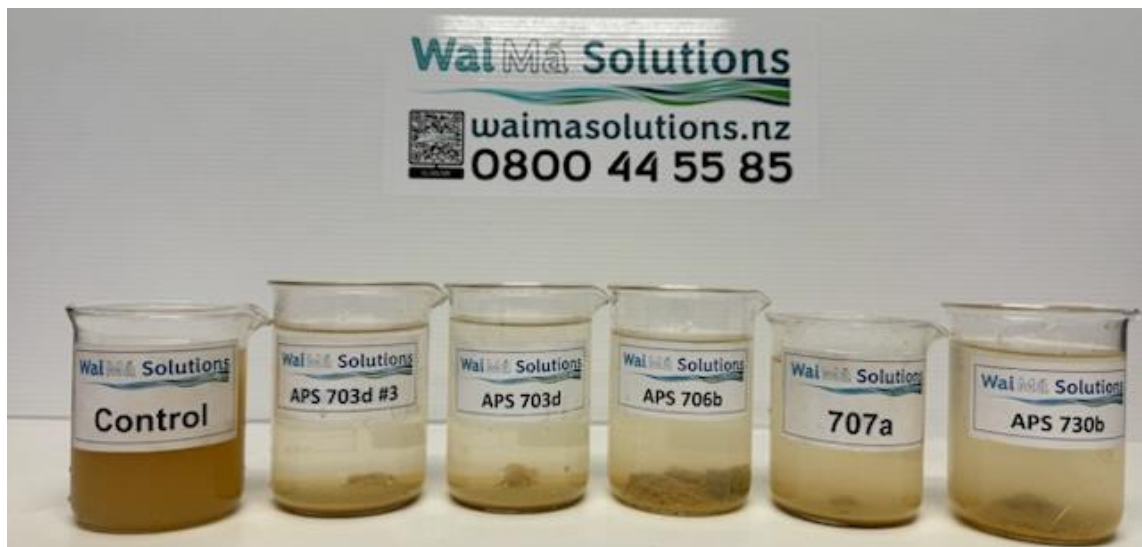
Figure 8. TP224 Bench testing results of Flocculants.
